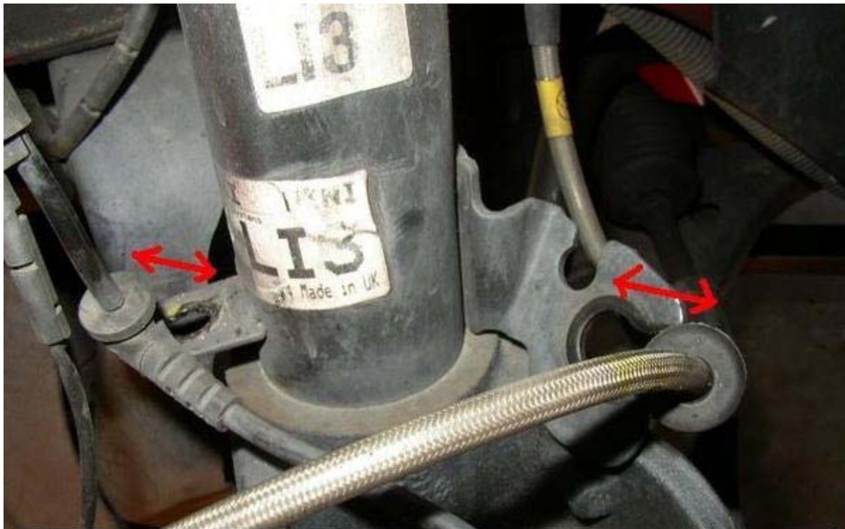
Front - remove brake line and wire from shock
