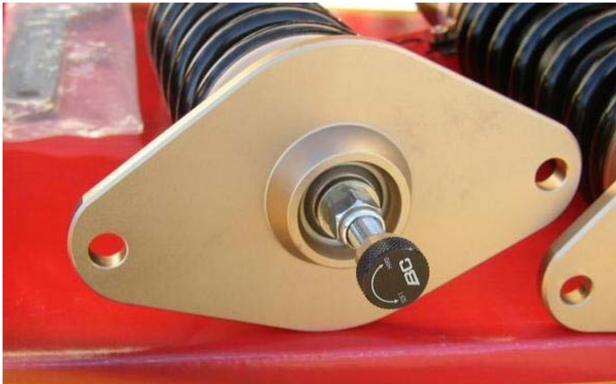
Rear top view. 30 way adjustable compression / rebound
