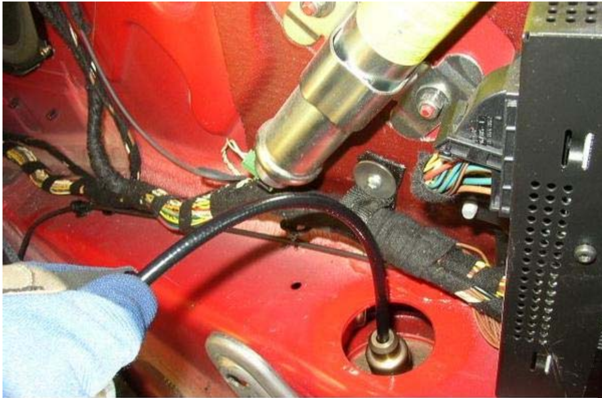
Flexible extension attached to the adjustor. You DO NOT ! HAVE to run this.
