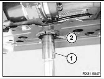
Position hydraulic gearbox jack (1) at jacking point (2) on chassis subframe.
