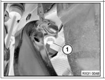
Undo centre bolts (1) for left and right chassis subframe at vehicle body. Tightening torque 31 11 1AZ.
