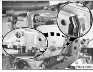
Make sure fluid strainer is correctly positioned on valve block.
