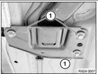
Release bolts on left and right 1 approx. 10 mm and lower chassis subframe.
