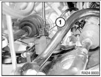
Disconnect headlight position sensor 1 (depending on equipment).
