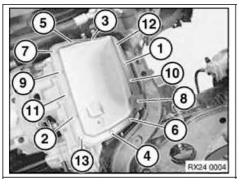
Unscrew fluid sump mounting bolts in specified sequence (13-1) and remove fluid sump.
