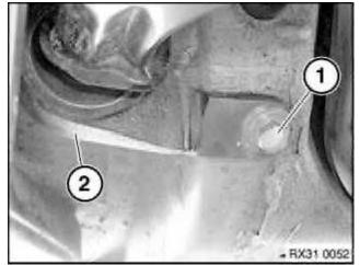
Remove bolts (1) holding the housing of rubber mount (2) at the left and right on the car body.
