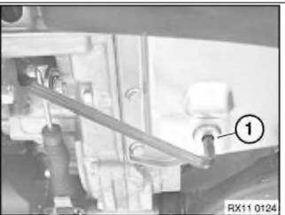
Remove oil drain plug 1 from transmission sump.
