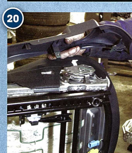
20 Remove the plastic side covers for the seat base. The rear plug on each cover was removed in step 18. There are two clips left to detach
