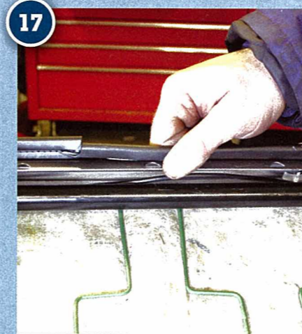
17 Turn the seat over and unclip the seat base cover at the back. This is secured with a long plastic u-shaped clip and will probably break in places
