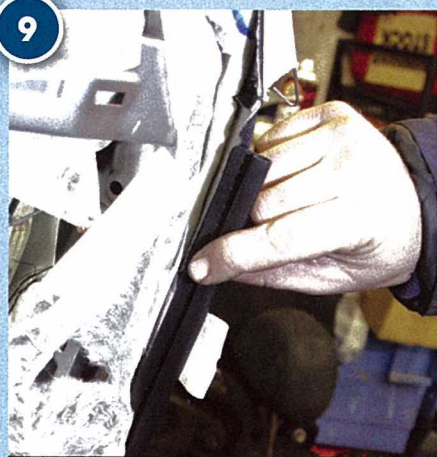
9 Unclip the side of the seat cover where the airbag is fitted. This is retained with the same type of u-shaped plastic clip as in step 6
