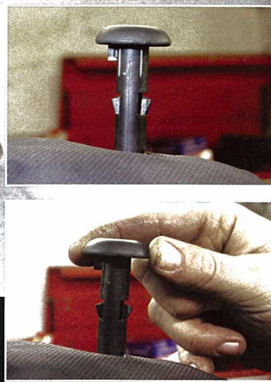
11 Pull the seat back cover up off the seat frame. Use a thin screwdriver to push the clips in for the headrests (two for each leg) and pull out the plastic sockets
