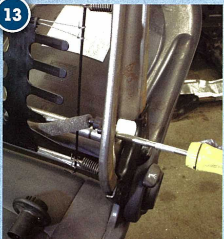
13 Pull the plastic cover off the lumbar support lever. Undo two Torx T20 screws to remove the lumbar support mechanism. Unhook the four springs for the lumbar support webbing
