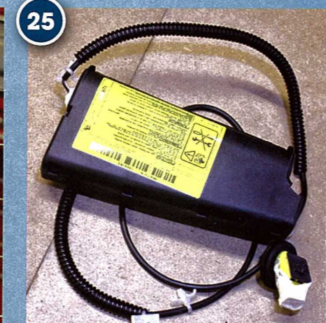
25 Place the airbag aside and cover the end of the yellow plug with masking tape. If static electricity causes a short circuit across the plug's contacts, the airbag could be activated
