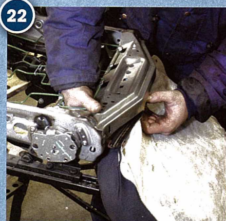
22 Pull the seat base cover forwards and detach the front of it from the seat frame. It's retained with a full length u-shaped clip
