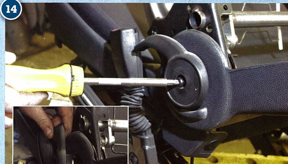
14 Tilt the seat fully forwards. Undo the Torx T30 bolt in the centre of the recline lever, then remove the plastic lever
