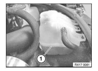
Continue topping up coolant in expansion tank to max. level (1). Start engine and run at idle speed.
