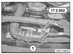
Release spring strap on lower coolant hose (1) with special tool 17 2 052  $\,$  .
