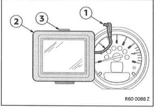
Connect the cable (1) to the navigation device (2).
