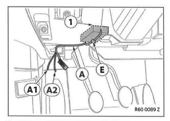
Route the wiring harness of navigation device mount **A** along the steering column of the existing standard wiring harness behind the dashboard.
