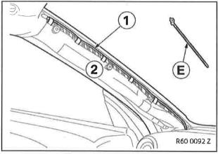
The airbag function must not be adversely affected by the cable routing. ◀
