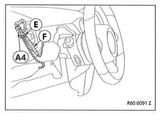
Only with the optional installation of the TMC aerial for 3.5" navigation device or where the navigation device is converted from 3.5" to 4.3" Connect TMC aerial F to branch A4 and secure with cable tie E. Route the aerial cable from TMC aerial F to the A-pillar.
