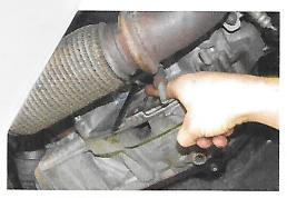
Step 1: Remove the right-hand wheel arch trim to access the crankshaft central bolt.
