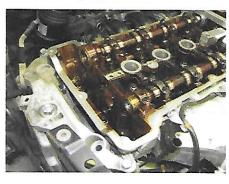
Step 8: Assemble the new timing chain rail cassette with the new crank sprocket held in place with the specially designed tabs.
