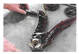
Step 2: Remove the chain tensioner and collect the residual oil with a shop towel.
