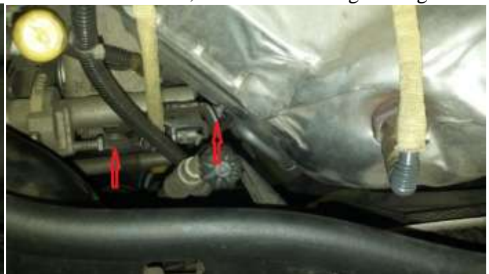
Loosen left bolt, rotate bracket to get to right bolt
