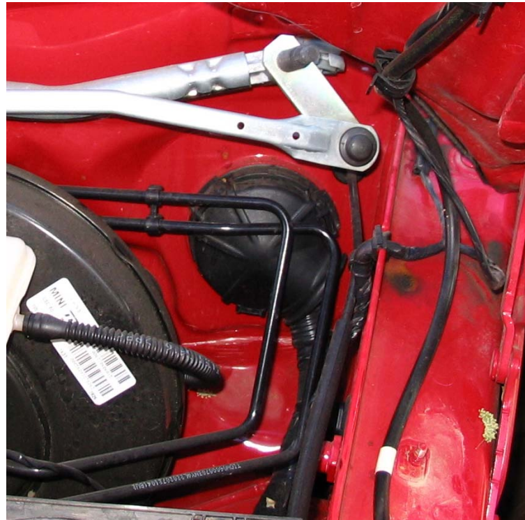
Here's the grommet and cover that the wiring harness comes through.
