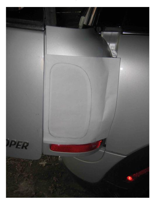
You only really need one of these tracings. The left and right openings are mirror image identical. Reversing the template will allow fabrication of the other trim ring.
