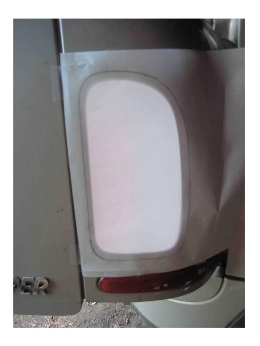
I do not have a photo of my process of marking the ring in pencil. But it is done with a standard sharpened wooden pencil laid crosswise( the way you might make a gravestone rubbing image) and creating a trace of the crease/ridge. This plastic molding is pronounced enough to easily create a sharp duplicate pattern on the tracing paper.
