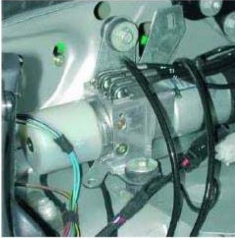
Hydraulic Unit Mounted
