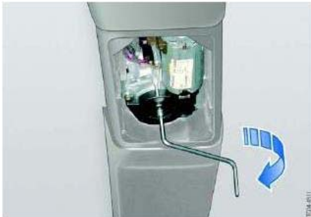
Fig. 16: Turning Hexagon Wrench In Clockwise Direction Courtesy of BMW OF NORTH AMERICA, INC.
