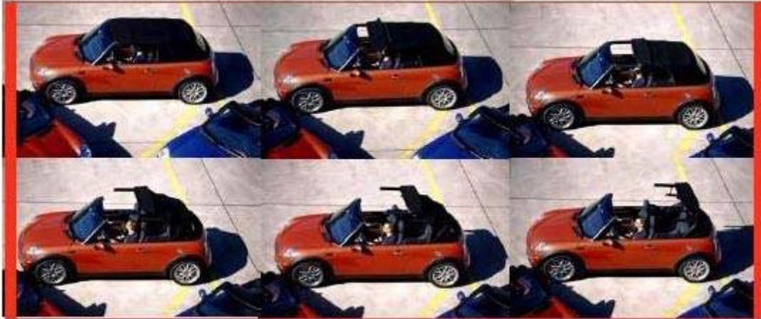
Fig. 13: Convertible Top Operating Principle Courtesy of BMW OF NORTH AMERICA, INC.
