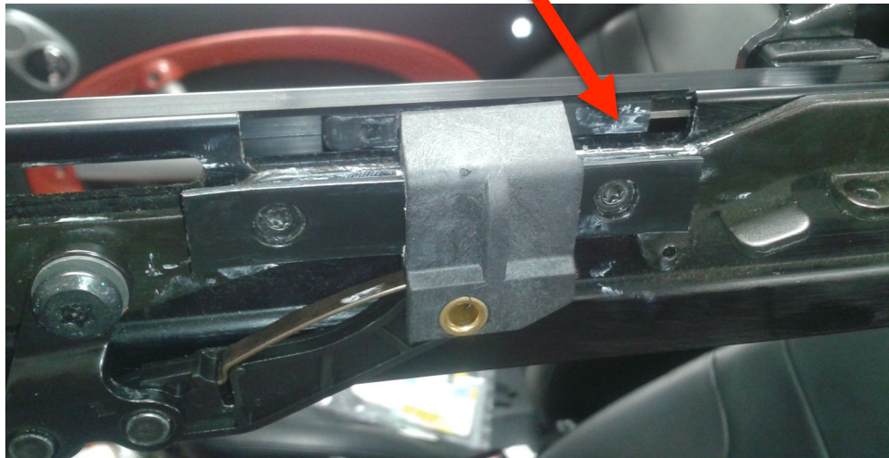
Front end of latching hook actuator rod
