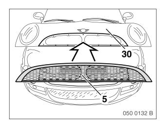
Secure the accessory radiator grille (5) to the bonnet (30) in the same way as the standard radiator grille.
