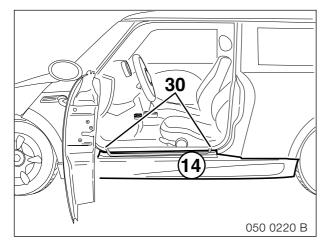
As you secure the accessory side skirt ensure that the adhesive tape is affixed to the complete area with uniform pressure.
