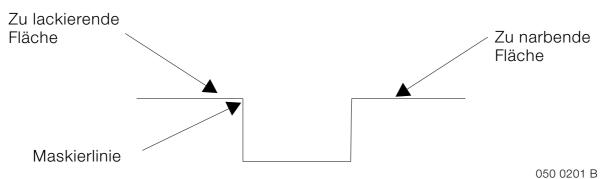
The figure shows a section through the component and masking joint.
