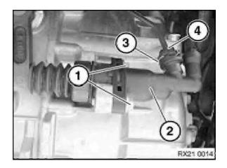
Release screws (1) and remove clutch slave cylinder (2). Remove clip (3) and disconnect line (4).
