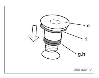
Screw in the stud bolts (e) with the appropriate spacer washers (g, h).
