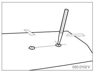
Gently centrepunch all eight holes through the templates. Remove the templates. Mask the working area to protect it.
