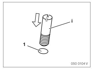
Enlarge the hole (1) to 10 mm using a step drill or peeling drill bit.
