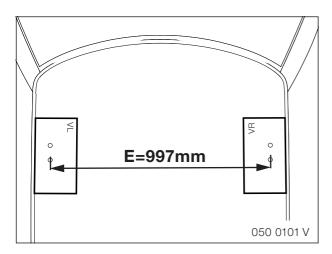
Check that the distance between the VL and VR templates is  $\mathbf{E} = 997$  mm.
