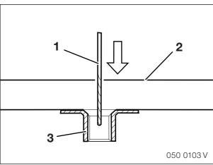
Predrill the holes with a diameter of 3 mm.
