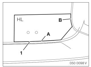
Place the cut edge (A) of template HL on the roof strip (1) at the rear left of the roof.
