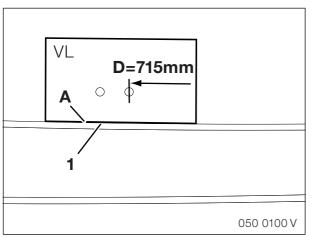
Place template VL at the marked distance  $\mathbf{D} = 715 \text{ mm}$  from template HL with the cut edge (A) on the roof strip (1) at the front left of the car.
