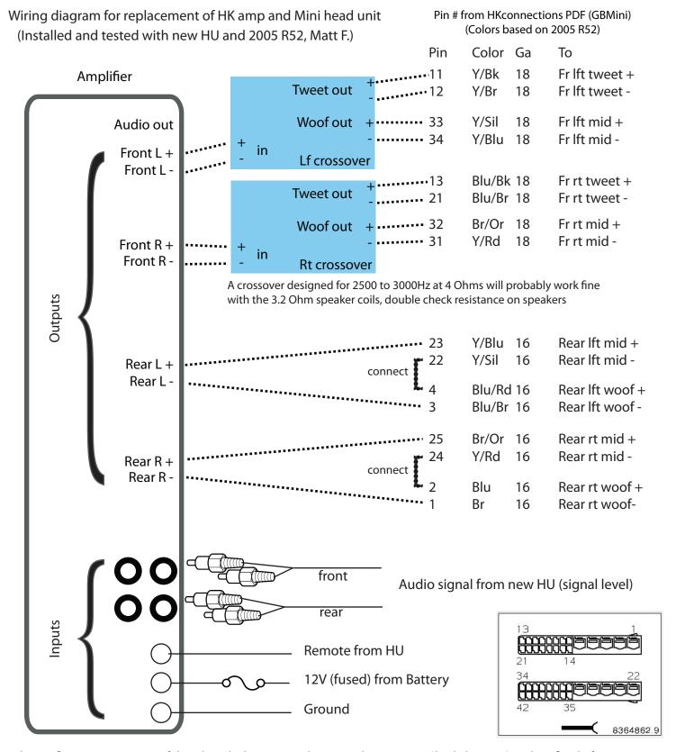
Note: This configuration was successful on the vehicle mentioned, your results may vary. Check the pin #'s and confirm before turning anything on. You can also test the speakers for resistance to confirm that they are in fact speakers.
