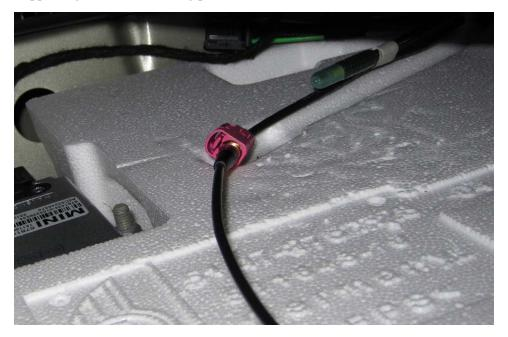
Route the extension cable out the left side of the box (so it can easily be threaded to the front console later) and screw the box back into place.
