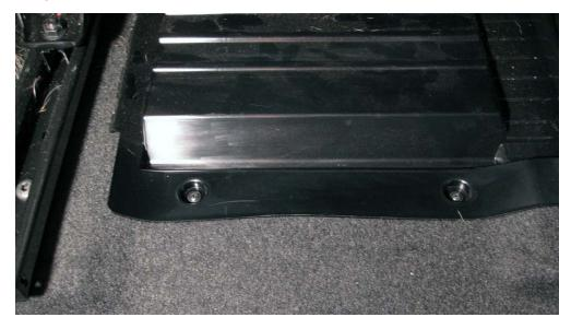
Remove the two screws shown in the picture above.
