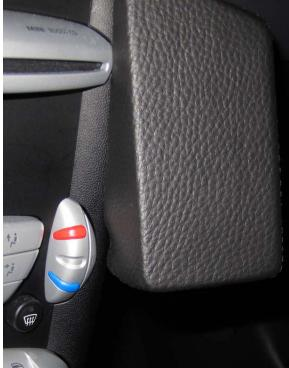
The result was the Kuda just *barely* cleared the opening glove compartment door, did not interfere with the temp switch operation, and was held firmly enough in place by the screw into the console and tab into the CD bezel area.
