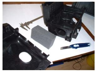
Mark where to cut and hold the whole foam block down with a wooden board. Cut the piece of with a very sharp knife or cutter. Release the foam block and you have a perfect cut.
