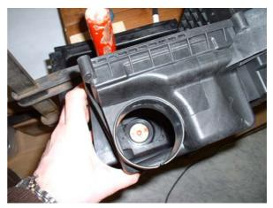
Drill gently two times through the cowl as done before through the air filter box by using the holes in the wooden board as guidance.
