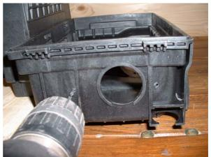
Using them, the lower part of the air filter box is temporarily fitted to a wooden board with two head wood screws. The wooden board will give a proper guideway for the core bit. Fixing the wooden board to your workbench makes it easier.
