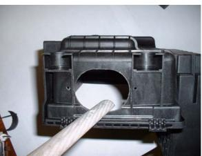
second one is located on right hand side. This is correct as we are looking at the front of the partition cowl, whereas we were looking at the of the lower part of the air filter box previously. Ensure that the wholes for guidance are in parallel to the lower end of the cowl. Double check it fits, by holding the box in front of the cowl and look through the front opening.
