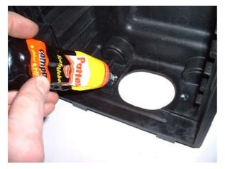
Apply contact glue like pattex to the front side of the partition cowl and the relating side of the foam block. Wait for 5 - 10minutes as instructed for the glue. Stick the foam on the partition cowl. It must fit at first try! Press it together hardly once, that's it.
