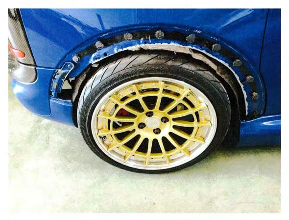
As you can see from the pictures, you need to cut metal 0,5cm off the holes for standard wheel arches.
