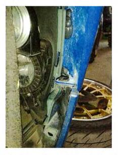
Fibreglass arches are more rigid than plastic bumpers: that's why particular attention has to be put on bonding and sealing the corners of wide arches which link with the bumpers' corners. If those corners tend to stay "up" from bumpers, just get a heat gun and heat them gently and gradually to soften them and take shape onto the bumpers, then keep them in place with American tape and/or spring clips while glue dries out (see picture below).
