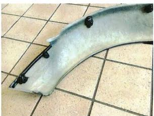
Place double sided tape 1 mm below the edge of the perimeter of the arch, only where you see the track for bonding (on rear arch you will put tape on the whole perimeter).
