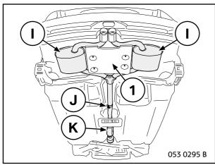
Install the John Cooper Works exhaust system I, J, K accordingly. The welded brackets on the John Cooper Works rear silencer I should be secured to the standard mounting fixtures.
