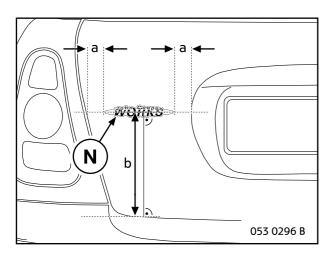
Adhere the double-sided adhesive tape to the back of the John Cooper Works emblem **N**. Use benzine to clean the adhesion surface. Determine the position of the John Cooper Works emblem between the hatch and licence plate mounting.
