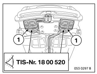
Completely remove the standard exhaust system
