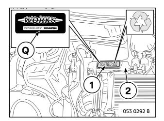
Remove original MINI emblem 1 from valve cover 2 and then clean adhesion surface with benzine.
