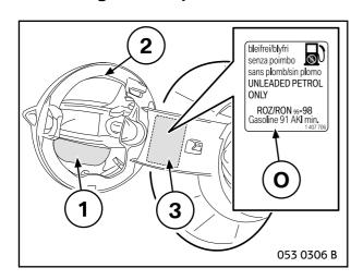
Remove original sticker 1 from the fuel filler cap 2. Use benzine to clean the adhesion surface 3.
