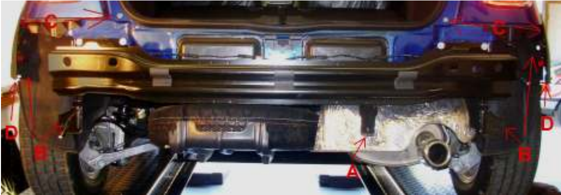
Picture 2 – Rear Bumper off (same locations for Cooper and Cooper S, this is a Cooper)
