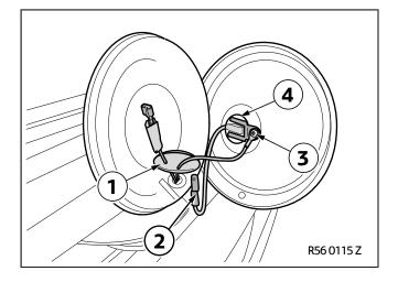
The tightening torque for the screws is 12 Nm.
