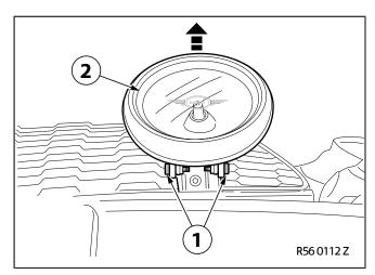
Unscrew both screws (1) and pull the additional headlight (2) carefully forwards.
