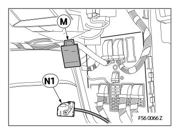
Connect branch **N1** to interface **M**. Secure interface **M** at a suitable point.
