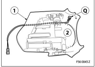
Route the cable from button **Q** below the foam insert of the steering column trim lower section (1).
