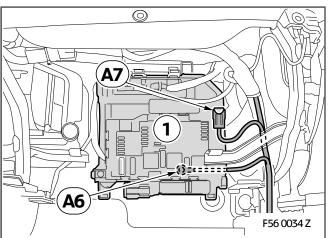
Release the fuse box (1) and place it to one side.
