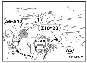
To ensure a good ground connection, remove any paint from ground support point **Z10\*2B**.
