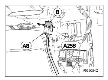
Connect control module B to branch A8.
