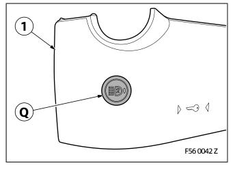
Clip button **Q** into the steering column trim lower section (1).
