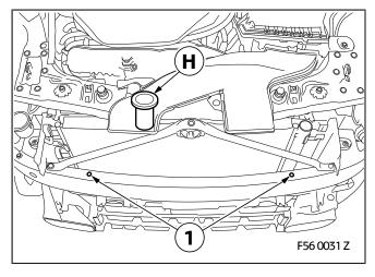
Drill through the holes (1) with a 9.1 mm diameter drill bit.
