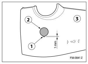
File out the cut-out (1) on the drill hole (2) as per the dimensions on the steering column trim lower section (2).
