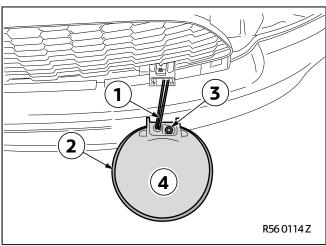
In order to avoid damaging the cable (1), hold the additional headlight (2) with one hand. ◀
