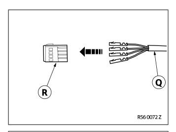
Connect the branches of button **Q** as follows to socket casing **R**:
