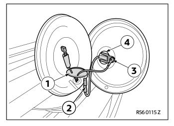
The tightening torque for the screws is 12 Nm.
