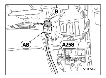
Connect control module B to branch A8.
