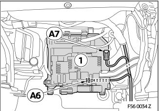
Release the fuse box (1) and place it to one side.
