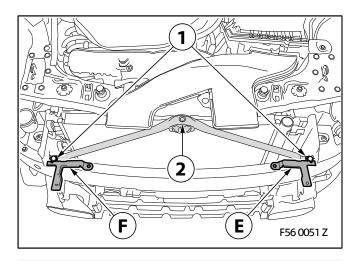
Unscrew the screws (1) on the reinforcing strut (2).
