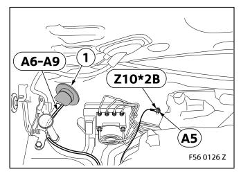
On RHD cars, screw branch **A5** to the negative terminal of the car battery.
