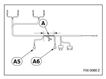
Wind up the cable around branch **A5** and **A6** of retrofit wiring harness **A**.
