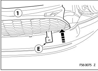
Push bumper trim (1) over additional headlight bracket **E** but do not secure into place yet.
