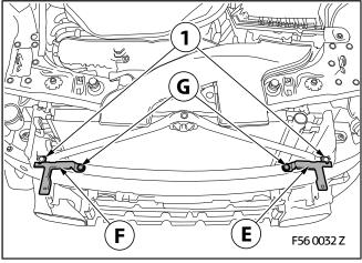
Screw on additional headlight holder **E** and **F** using pan head screws **G** and original screws (1).
