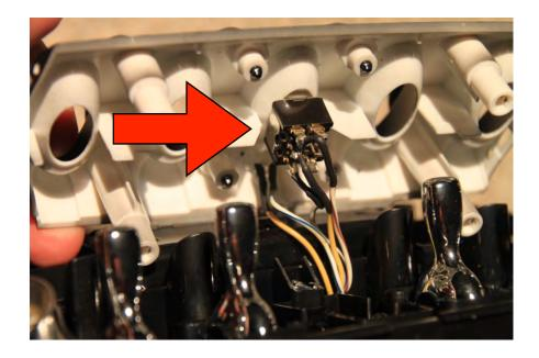
I used the chrome cap from the ball point pen, using JB Weld to attach it to the mini toggle switch. The cap I used slid onto a plastic tube on the pen, I glued a piece of the tube onto the switch, then attached the cap.
