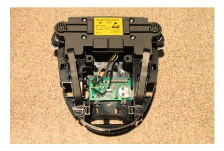
I unsoldered the LED from the circuit board and installed it in front of the switch bank, drilling a small hole and holding it in place with hot glue.
