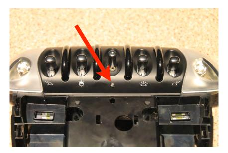
I had to cut away the plastic where the sunroof switch would normally mount to make clearance for the mini toggle switch, I also drilled a hole for the wires to pass through to the circuit board
