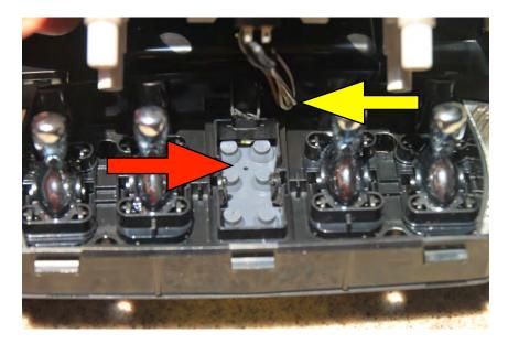
I drilled a hole in the sunroof switch blank and mounted the mini toggle switch.
