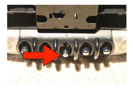
I ran wires from the toggle switch to the circuit board, there was a common point for the two buttons (circuit board) that went to the center post on the mini toggle, the line for each of the buttons went to one of the outer posts on the mini toggle.
