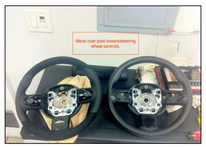
9. Now it's time to install the new steering wheel. Before you do that, take time to notice the slot in the bottom of the steering wheel shaft. This is designed to make sure that the steering wheel goes back on in perfect place and the steering wheel is properly lined up.
