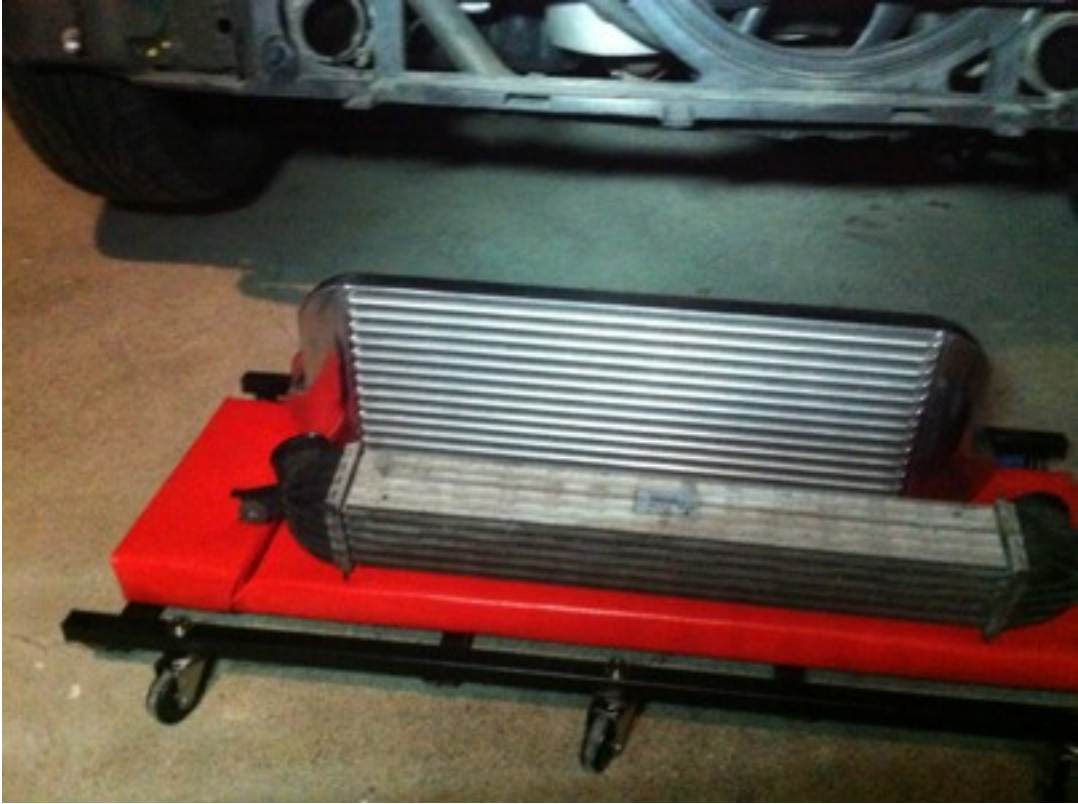
HERE IS THE HELIX INTERCOOLER AND THE OEM INTERCOOLER...
