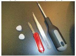
1. I removed the visor from the car using a thin pocket knife. I found that if you push at least 1/4" in and then try to pop out the screw cover it does not hurt the plastic. CAUTION! After unscrewing the visor do not forget that it is attached to wires for the visor lights. Gently pull down and then unplug the visor.
