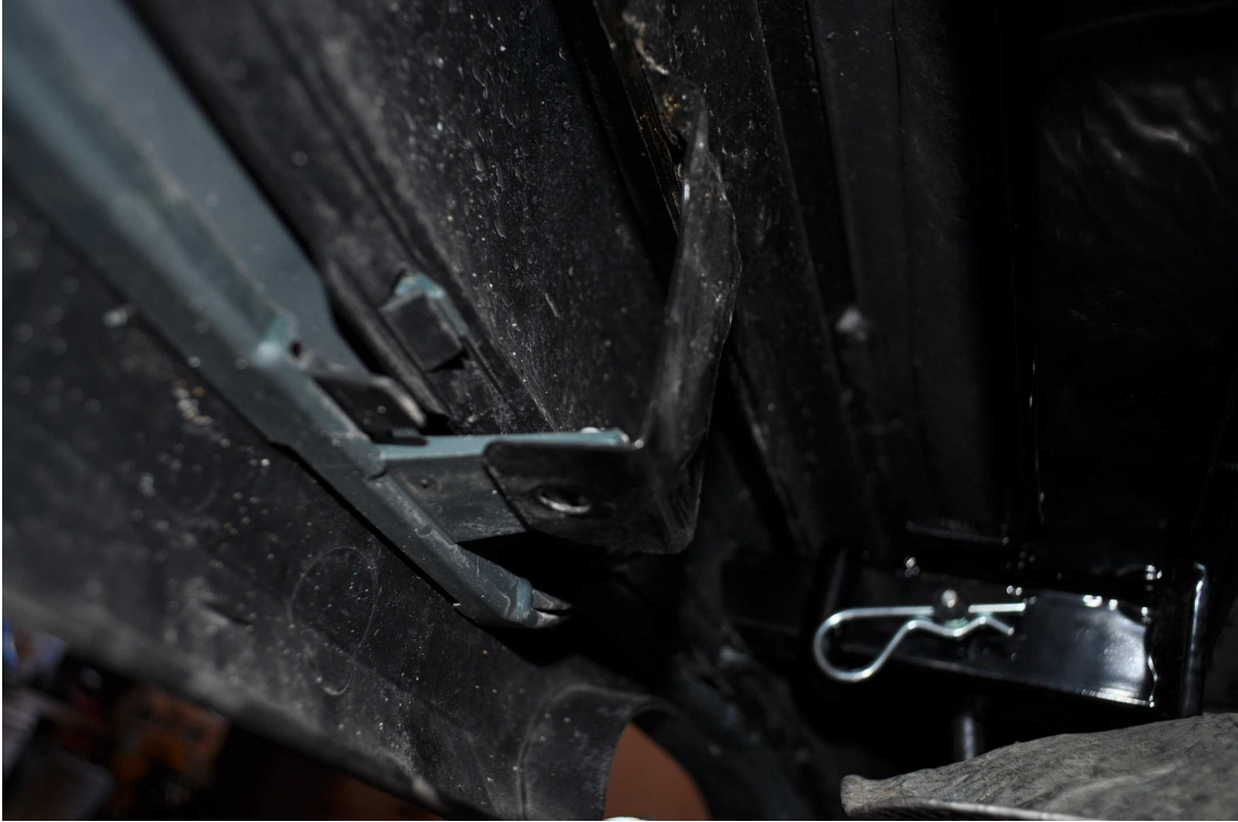
Here is a shot under the bumper showing the hitch pin in place and the fact that I hadn't put in the last bumper fastener yet.
