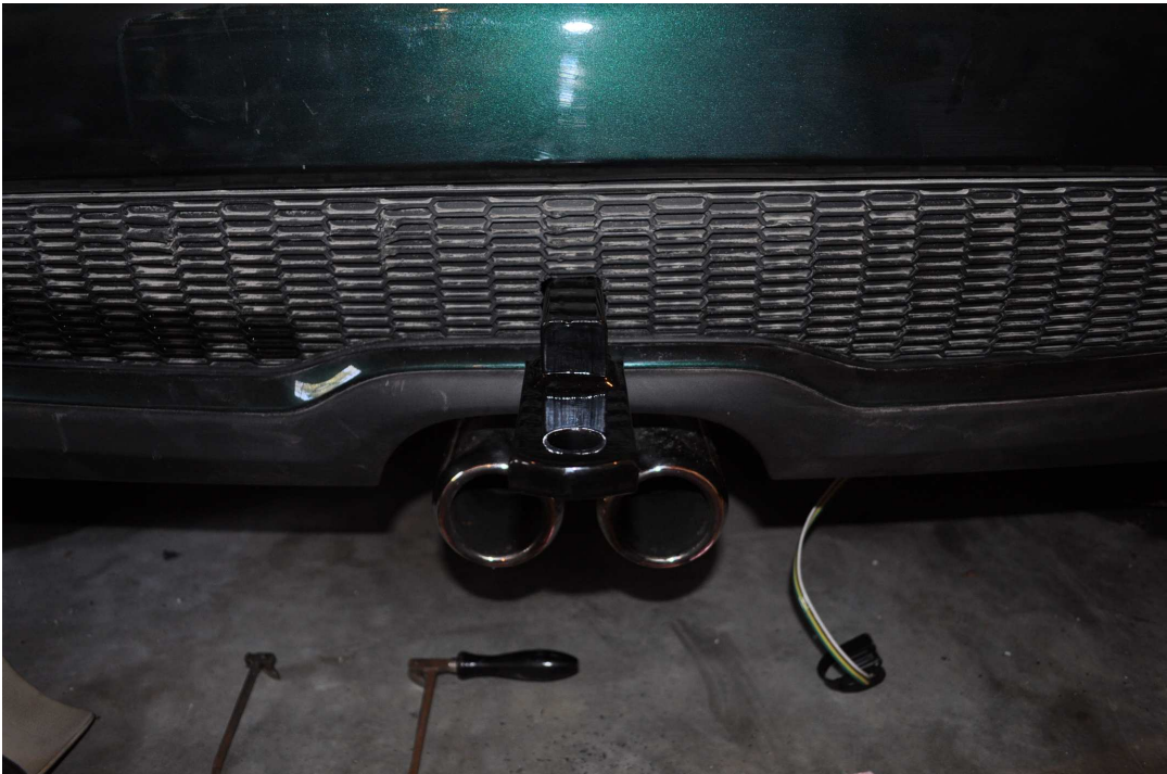
Shot of the bumper with the hitch in place and trailer lighting wire. I figured out I could use the cap cover for the trailer converter (I didn't end up using the coping saw that's seen on the floor)
