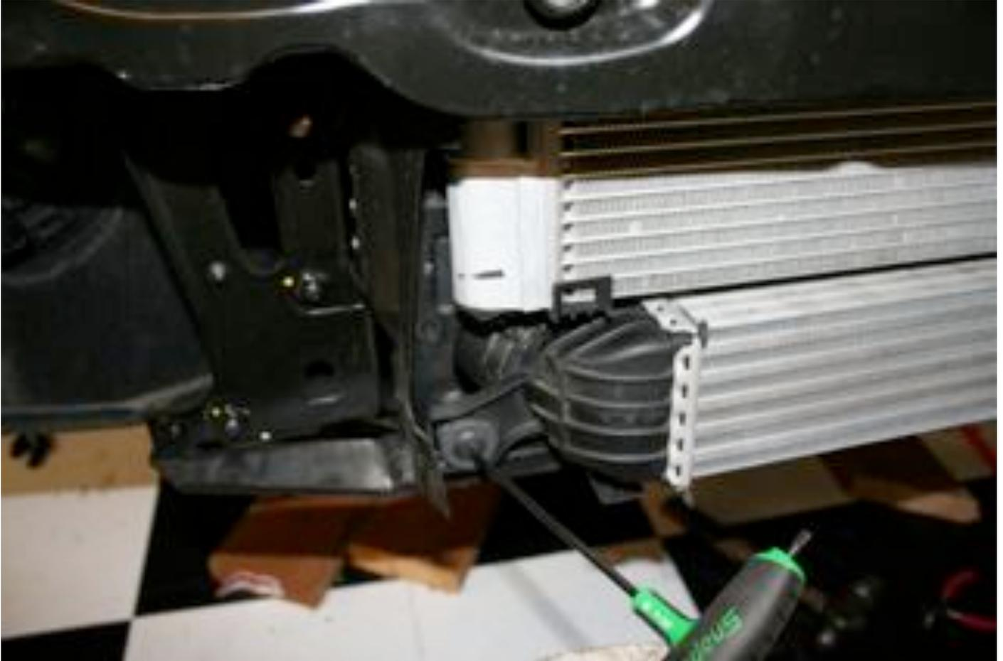
12) Trimming plastic to gain extra clearance. The next series of photos shows before and after trimming on both sides of the intercooler. This is important to allow enough clearance to the new ALTA Core. You really can't trim too much, but you do need to avoid removing the OEM mount areas, so you can re-install the OEM core if you choose to in the future. Driver side first:
