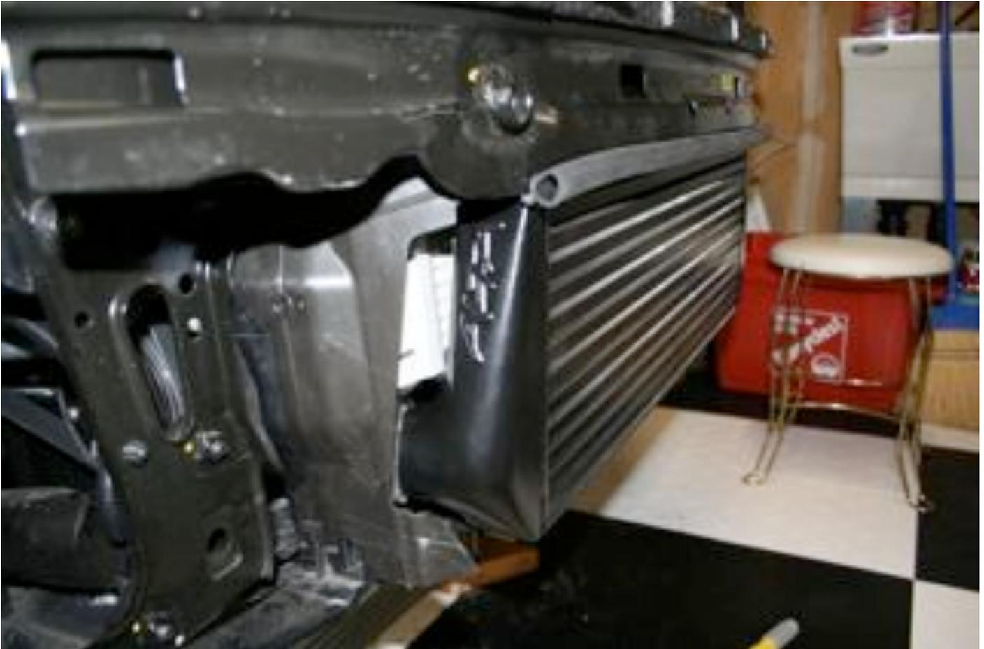
14) Now lets trim the bumper! The following pictures show what and where to trim off the back side of the bumper. Please note you must remove the temp sensor from the bumper. You will remove its mount. Then wire tie it back into a similar position. (NOTE: BEFORE is shown first!)
