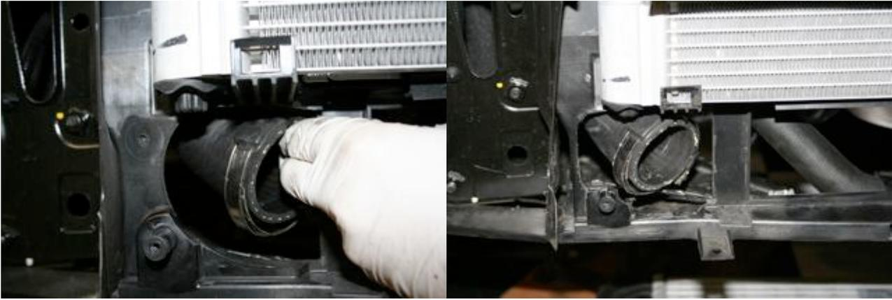
13) I did forget one picture and I am sorry but the photo shown below with the core mounted gives you the right idea. You need to file back the little plastic stays for the IC condenser shown in the photos above. They need to be slimmed down a bit to allow the ALTA core to rest farther back. Once that is done place the supplied rubber trim over the bottom side of the bumper beam to help cushion the core. Then install the core and tighten the clamps.
