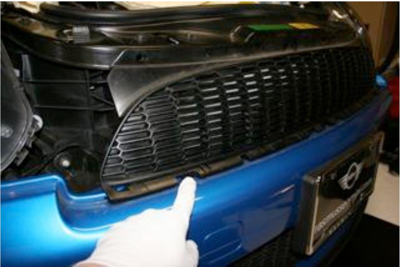
5) Now remove the TORX screws that are now visible on both sides of the bumper. Shown below with my knee and tool.
