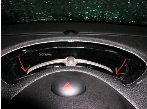
Now remove the plastic or wood trim located behind the steering wheel and tachometer. To do this, I lowered the steering wheel all the way down and then I was able to get my fingers behind the trim and simply pull it off. With some creative maneuvering, it should slide out.
