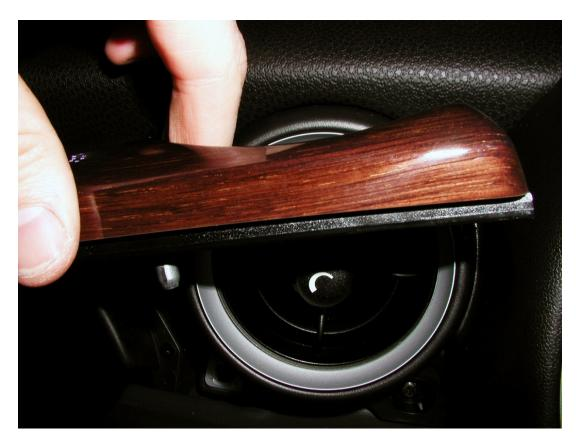
On the passenger side, open the secret compartment and pry out the plastic covers on either side (covering the vent screws).
