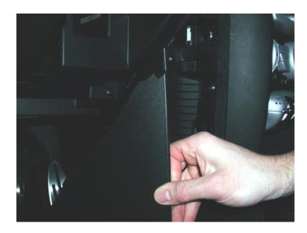
Now you will need remove the screws holding in the section of dash where your key inserts (4 screws) and the dash above the glove compartment (where the release button is—5 screws). The dash where the key inserts should just hang by the wire and the dash above the glove compartment does not need to come out completely, you just need to access the screws holding in the speedometer.
