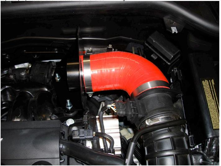
You are CLOSE to being done! Final tighten the mounting hardware for the air box. Then using the supplied trim, run it around the air box. Lastly install the filter. Use an old rag or paper towel to remove excess oil from the filter from the mfring process. Especially from the inside lip of the mounting surface. I use a light amount of simple green to help remove the oil in this area. Then slide it on, align the logo and tighten it.
