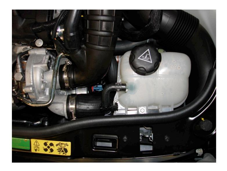
Now go under the vehicle and remove the two clamps that secure the lower portion of the tubing to the intercooler. Then remove the 90 deg rubber elbow from the bottom of the IC muffler. This is a snug fit so be patient. The photo below shows the upper clamp loosened. You can see in the right side of the photo, the muffler. This will be removed next.
