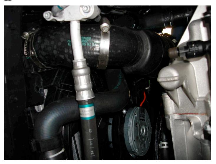
The photo below shows the lower elbow removed and the muffler still in place. Dead center in the photo is the PITA torx headed screw that secures the muffler to the radiator core. Find a way to loosen and remove this screw. Then the upper hose and muffler drop out the bottom as an assembly. Now on to the easy part!
