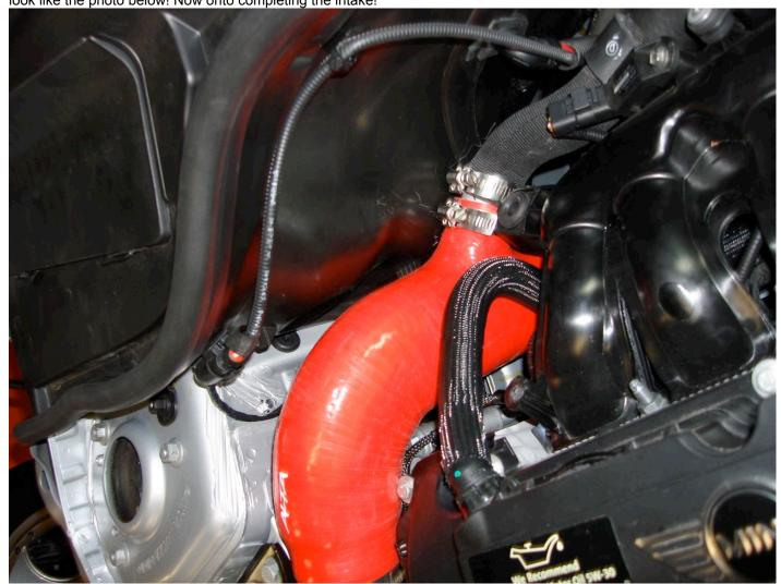
Mount the air box to the intake manifold using the supplied hardware. The hardware shown in the photo below WILL vary from that included in the kit, this is a pre-production hardware setup shown. Essentially the box mounts to the manifold re-using the OEM rubber cushions. The plate washers, bolts and nuts secure it through those mounts. Do not final tighten at this time.
