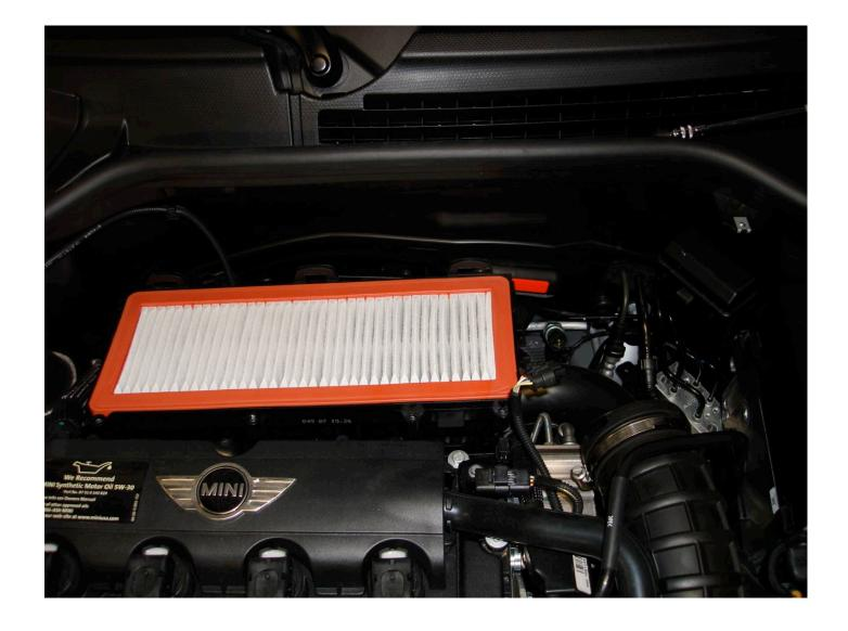
The photo below shows the air box removed and the cold side IC pipe still installed. On the lower left side you can see the clamp securing it to the plastic boost tube. Loosen this clamp. Then loosen the clamp near the firewall that secures the sound generator recirc hose to the boost tube. Once loosened then remove the hose from the boost tube and tuck
