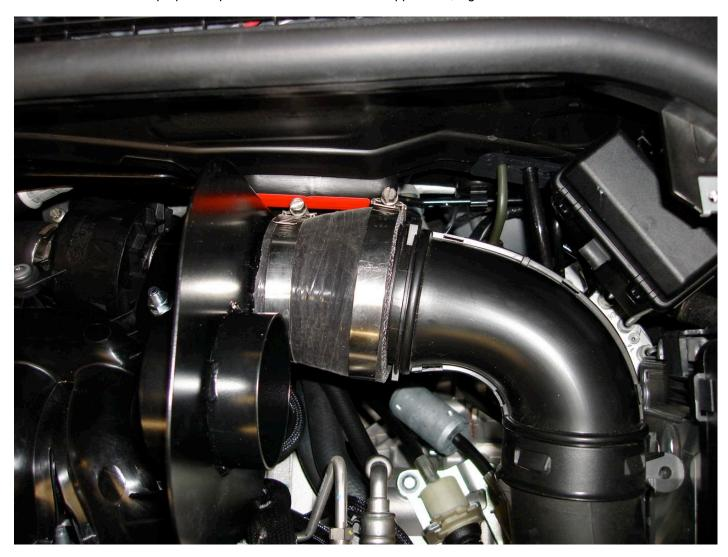
Now install the MAF sensor into the ALTA upper tube and secure with supplied clamp. Then carefully slide the sensor into the OEM inlet hose and then the ALTA hose over the upper tube of the air box. Tighten clamps. Again photo depicts a pre-production tube. Production versions have an ALTA logo.
