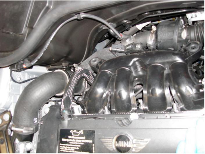
Then loosen and remove the clamp securing the tube to the T/B. This can be a bugger and may require a couple screwdrivers of varying lengths, or 7mm swivel sockets etc. Once that is off then remove the tube as an assembly.
