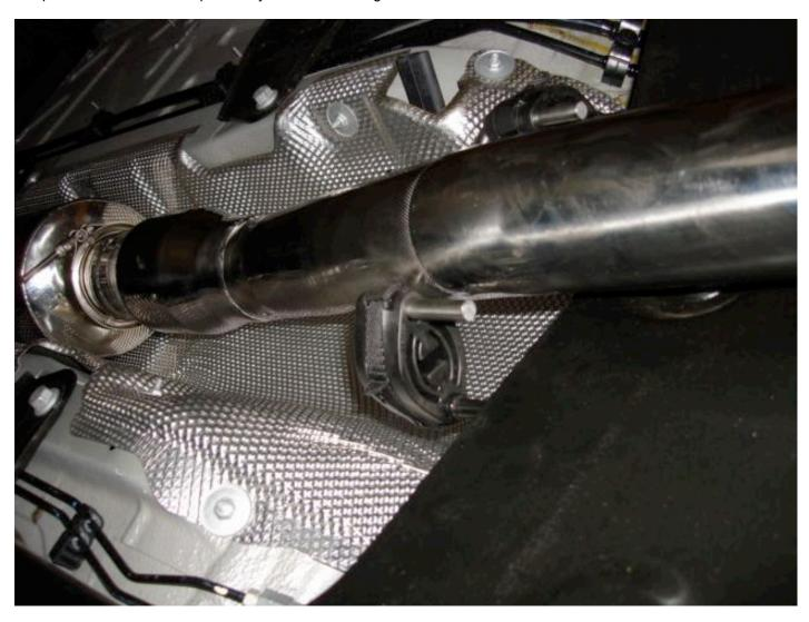
Now, be sure that all areas of the exhaust and downpipe are clear of other systems of the vehicle as well as the exhaust tips. Then final tighten the three bolts at the turbo and the v-band clamps to the torque specs printed on them.
