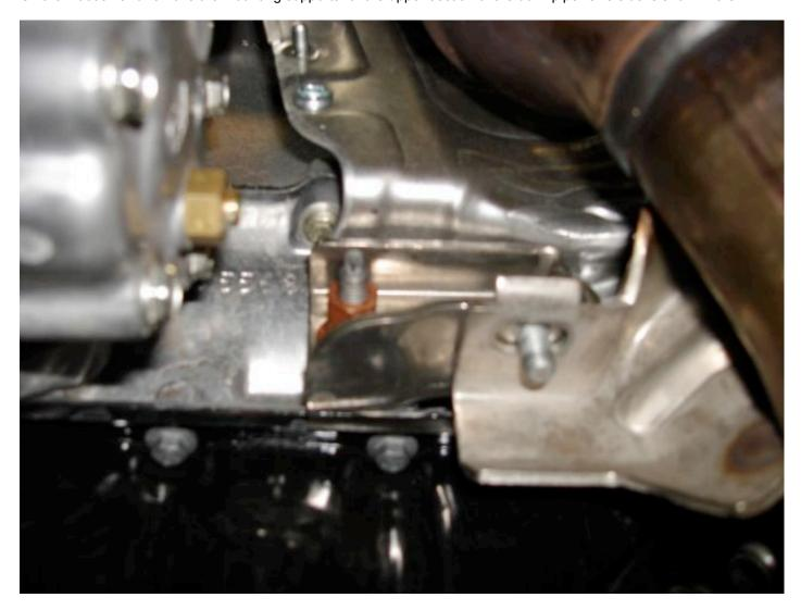
Now carefully remove the upper section and the remaining portion of the lower section. You will want to spray some lube again on the hangers as they can be a PITA to get the barbs past them without the lube! Now on to the fun parts!
