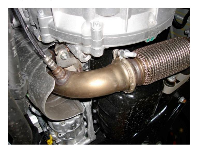
Ok then loosen and remove the mounting supports for the upper section of the downpipe. One side is shown here:
