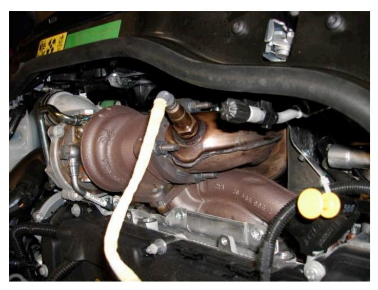
Then again grab the lube, and liberally douse the three mounting studs, nuts, front and back (seen above along with the O2 sensor prior to removal.) Let this set up for a while before attempting to remove them. This can be a real bugger if these strip inside the turbo housing. So be patient!
