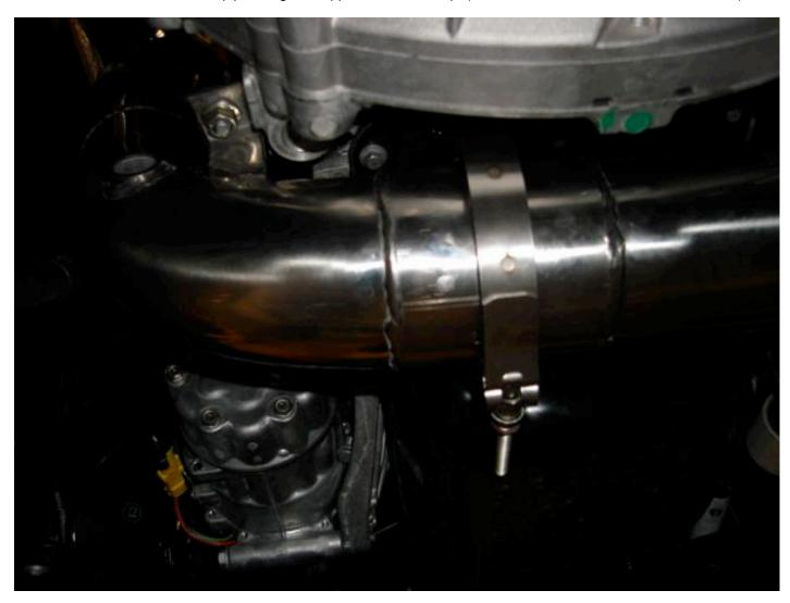
Then connect the DP to the exhaust. Again the next photo shows it being connected to the ALTA cat-back. Refer to the first photo of the removal sequence if you are connecting to the OEM cat-back.
