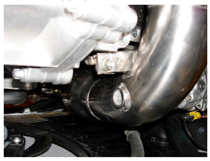
Then connect the lower section to the body by going through the hangers. After that loosesly secure the upper and lower sections of the ALTA downpipe using the supplied v-band clamp. (DO NOT FINAL TIGHTEN AT THIS TIME!)
