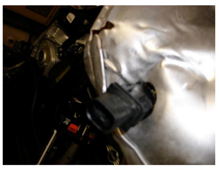
I simply used some tin snips to open the hole a bit. Then pulled the plug through. This may also aid in reassembly later on. (I also filed the rough edges to prevent cutting the shielding on the O2 harness wiring.)
