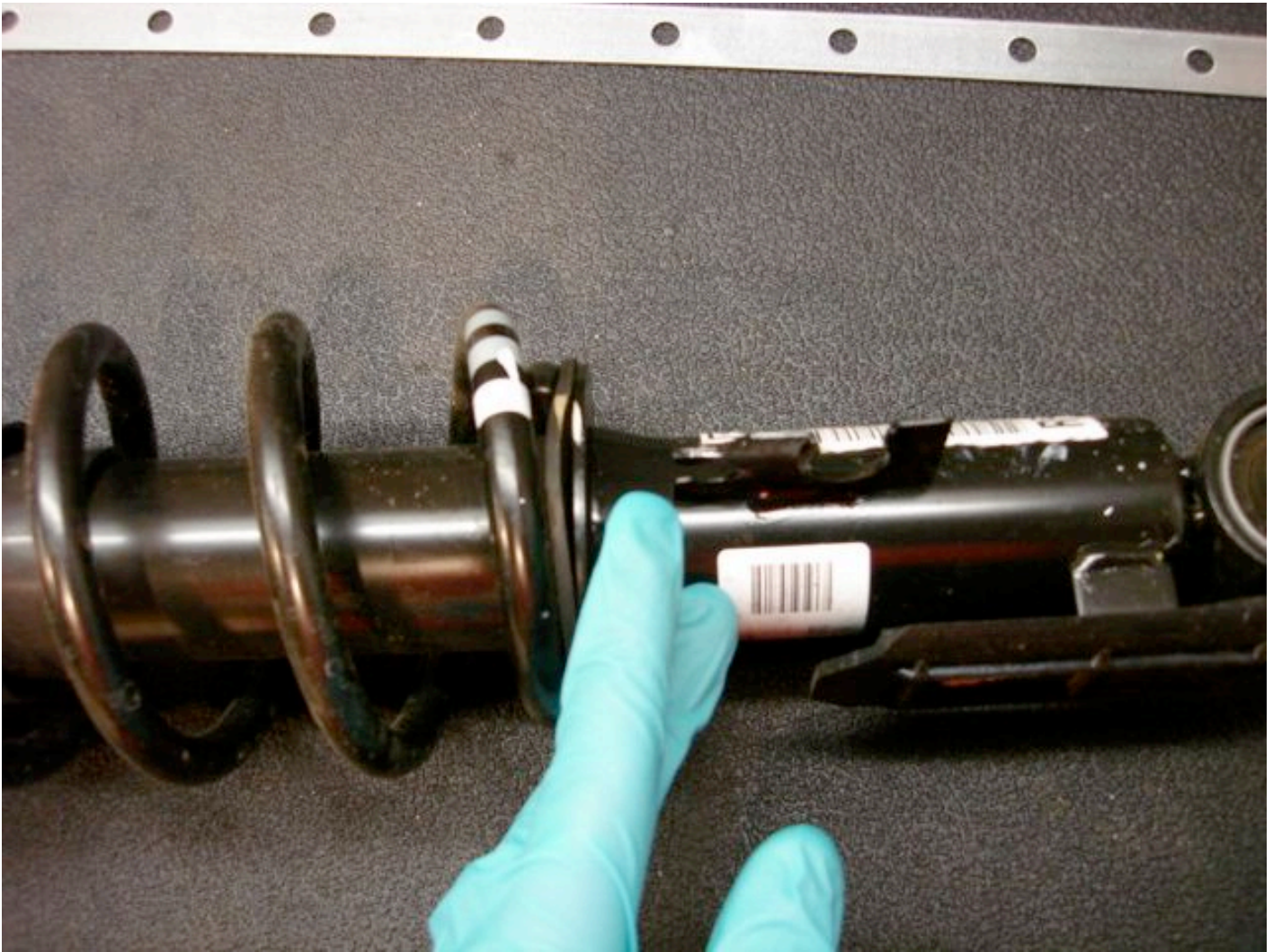
Now using a spring compressor (not shown) secure the spring. Or if you are a risk taker like me simply remove the nut on top using the allen wrench and combination wrench.
