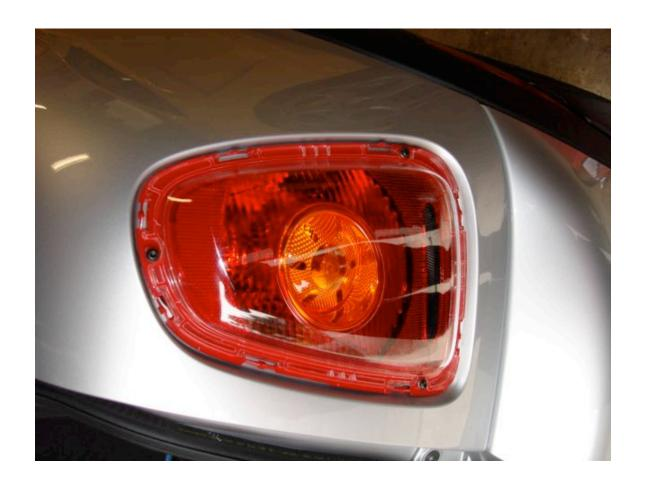
Then simply loosen and remove the three torx head screws that secure the lamp. Then working from in here with your hand:
