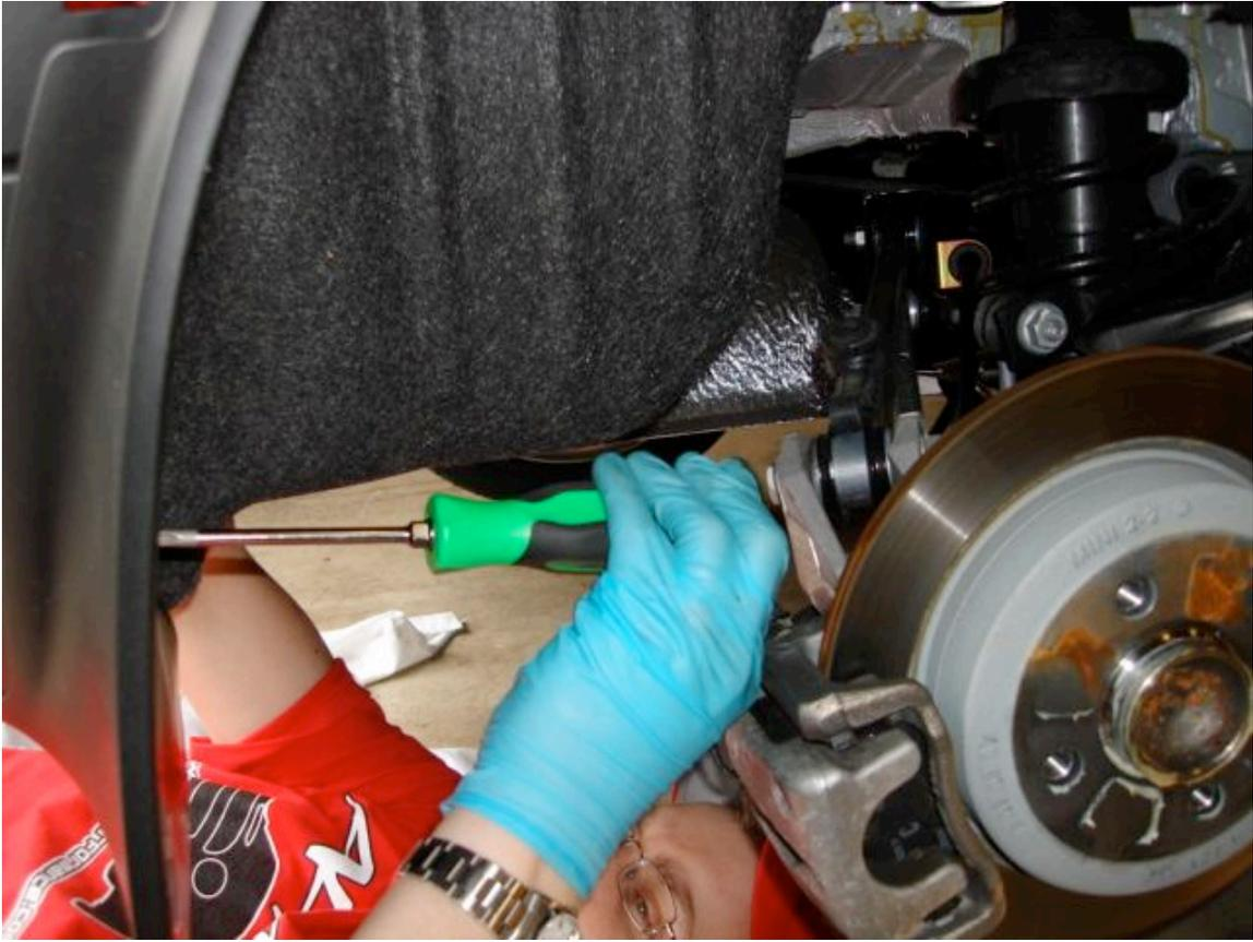
While holding the flap up and in position, use your bent awl to poke the other screw hole through the fender liner. Now again standing on your head, chewing gum and rubbing your belly attach the other screw. Like above don't tighten all the way.
