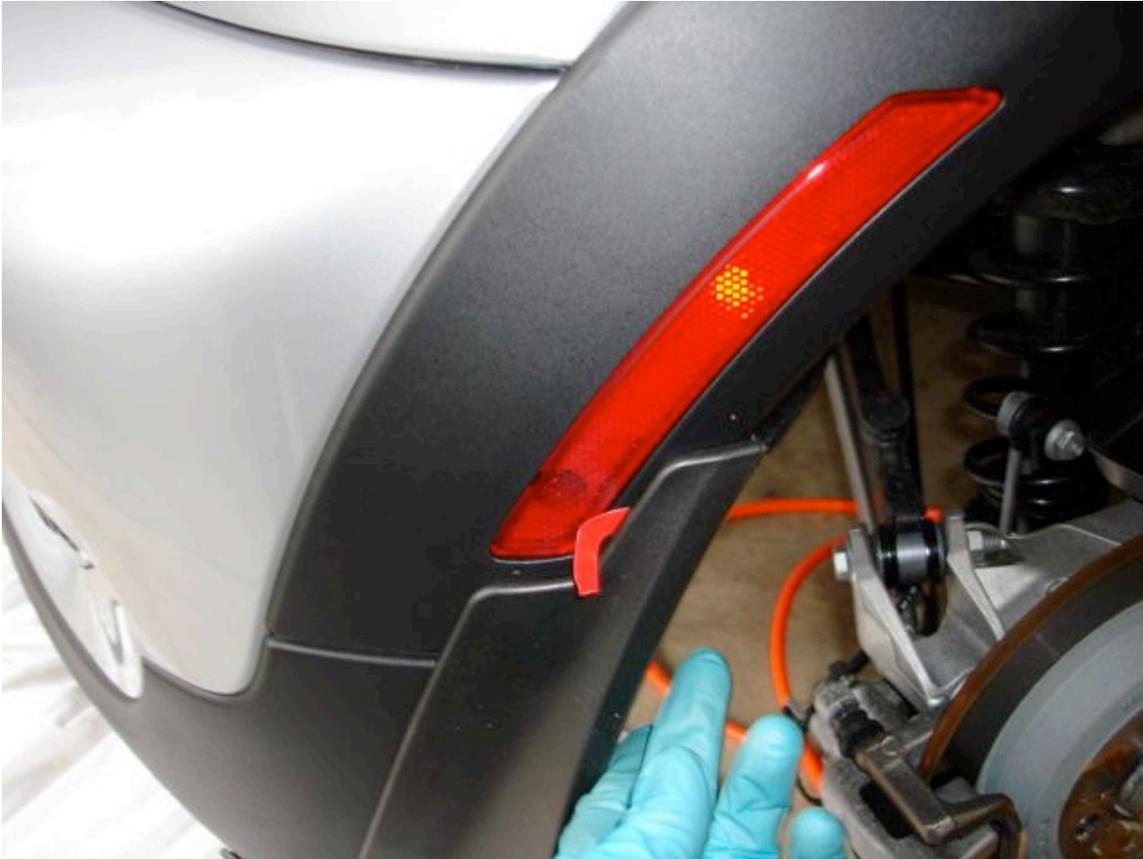
Then while simultaneously checking the alignment of the flap (and then when this side is done BOTH sides for symmetry) slide the retaining clips into the flap and over the fender trim (as like the front). This is best performed with a bent awl or flathead screwdriver, pliers and shop rags to prevent marring the surfaces.
