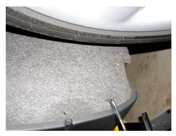
Then using the retaining clips as a guide, carefully trim the fender liner enough to allow each one to slip onto the liner and align with the holes made previously. I used a utility knife to make the necessary cuts. You don't have to be TOO particular as long as you don't cut a TON extra. Note below I have the upper installed and the lower trimmed.
