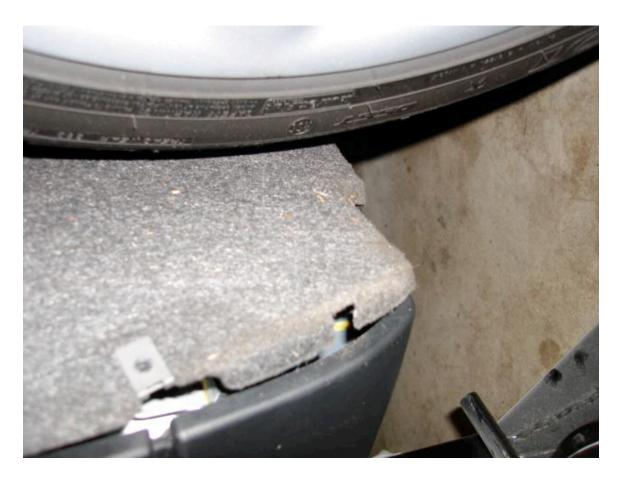
Next tuck the fender liner back into the fender. Then take the red adhesive release tape down and up approx. 1-2" each direction. DO NOT REMOVE all of it at this time!
