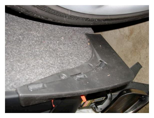
Pull the tabs of the release tape working out from the start point. The manual says use 5kg of pressure. I just pushed REAL hard and it seemed to stick. Then install the two screws to secure the inner fender liner to the flap.
