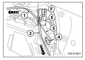
Connect the wiring harness **F** to the silencer receiver unit **E**. Route the long cable (1) from the wiring harness **F** using cable ties **G** to the front along the existing wiring harness into the passenger side footwell.
