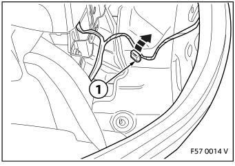
Take the cable clip (1) of the coarse thread stud bolt in the boot on the right-hand side of the car.
