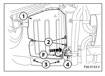
Reinstall the underfloor line (1). Tighten the three existing screws (2) for this purpose. Then secure the rear bumper trim in place using the two existing screws (3).
