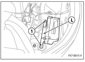
Push the fastening for receiver unit **L** onto the two coarse thread stud bolts (1) on the bodywork.
