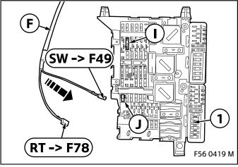
Connect the red cable **(RT)** from the wiring harness **F** to fuse plug **F78**. Insert the fuse **I** into slot **F78** (terminal 30B).
