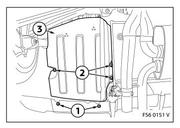
Remove the two screws (1) from the rear bumper.
