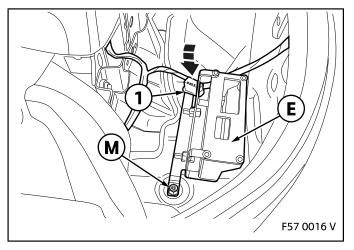
Attach the cable clip (1) to the coarse thread stud bolt on the bodywork.
