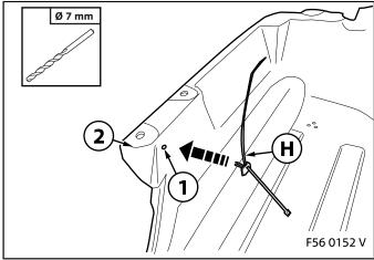
Drill a hole (1) with a **diameter of 7 mm** in the underfloor liner (2). Press the cable tie retaining bung into the borehole (1) along with retaining bung **H** from the inside. Secure the wiring harness **F** using cable tie **H** inside the underfloor liner (2).
