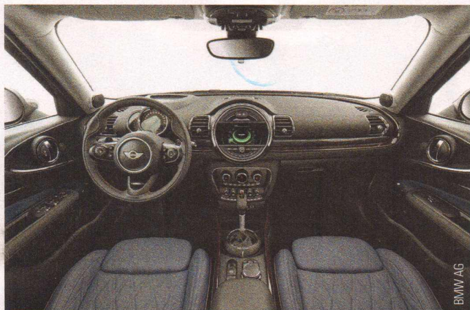
The central display is a standard 6.5-inch or optional 8.8-inch color screen for vehicle, infotainment, phone and navigation functions.
