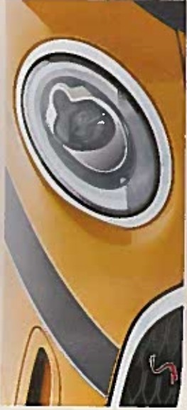
The optional white LED headlights provide both low and high beam and are surrounded by LED daytime-driving rings.
