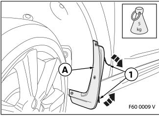
Pull off the tabs (1) and push the front mud flap **A** against the contour of the car several times.
