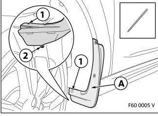
Position the front mud flap **A** and mark the boreholes (1) and (2) on the car using suitable tools.
