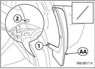
Position the rear mud flap **AA** and mark the boreholes (1) and (2) on the car using suitable tools.
