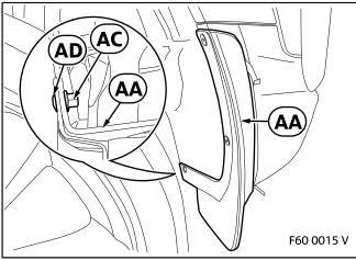
Place screw **AD** from outside through the borehole through the rear mud flap **AA** and secure it from the inside with cap nut **AC**.
