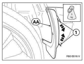
Pull off the tabs (1) and push the rear mud flap **AA** against the contour of the car several times.
