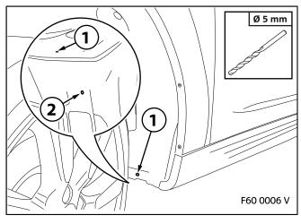
Remove the front mud flap **A** and drill holes at the marks (1) and (2) with a **diameter of 5 mm**.
