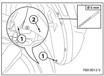
Remove the rear mud flap **AA** and drill holes at the marks (1) and (2) with a **diameter of 5 mm**.
