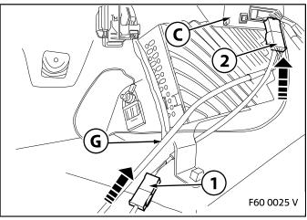
Connect the wiring harness **G** to the silencer receiver unit **C**.
