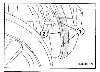
The areas being bonded must be completely dry, clean and free from wax or grease. ◀
