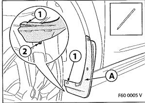
Position the front mud flap A and mark the boreholes (1) and (2) on the car using suitable tools.
