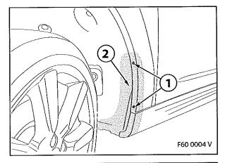
The areas being bonded must be completely dry, clean and free from wax or grease. • Remove the blind rivets (1) using suitable tools. Clean the bonding surface (2) with suitable products.
