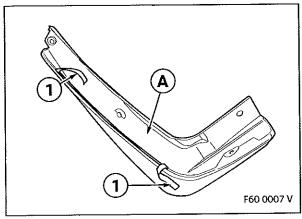
Bend the ends of the backing film (1) to the outside
