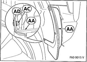
Place screw **AD** from outside through the borehole through the rear mud flap **AA** and secure it from the inside with cap nut **AC**.
