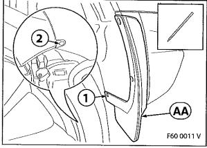
Position the rear mud flap AA and mark the boreholes (1) and (2) on the car using suitable tools.
