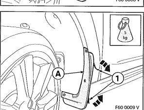
Ensure that all tabs (1) on the adhesive backing film are visible. ◀
