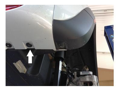
This picture is looking up under the same wheel opening. Again remove the indicated screw and set aside for assembly. Now use the cleaner first then the adhesion promoter on the area where the mud flap will go.
