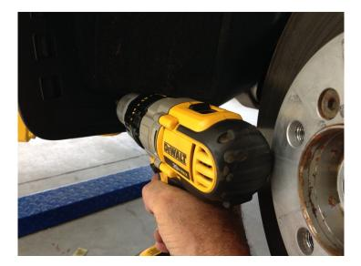
Last step is to install the self-tapping screws. If you have a right angle drill or battery powered driver it would make access easier, otherwise turn the steering in the direction of the side you're installing to get the most working room. The screws thread into the plastic of the wheel well trim and are the variety that drills their hole as well. A little force will get them started, but again no killer torque or you can strip them.
