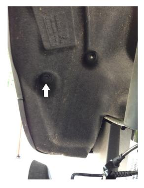
This picture is looking rearward into the passenger side rear wheel well. The arrow indicates which screw needs to be removed. Set the screw aside as it is reused when assembling the mud flap.
