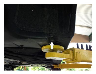
This is a photo of the front mud flap location, looking aft on the driver's side. The arrow indicates which screw has to be removed. Again set the screw aside as it is reused when assembling as before. Next install the clips in the same manner as done on the rear flaps.
