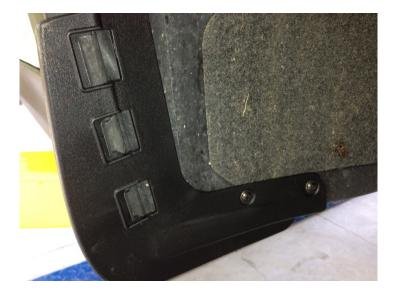
This picture shows the three clips in place on the front flap and shows the screws installed also. T hey clamp the mud flap to the flange of the wheel opening. I found this to be the most difficult part of the assembly. The clips are very strong and their opening is small. Here is where the large flat blade screwdriver comes in handy to push these into position using the flat side of the blade, not the end.
