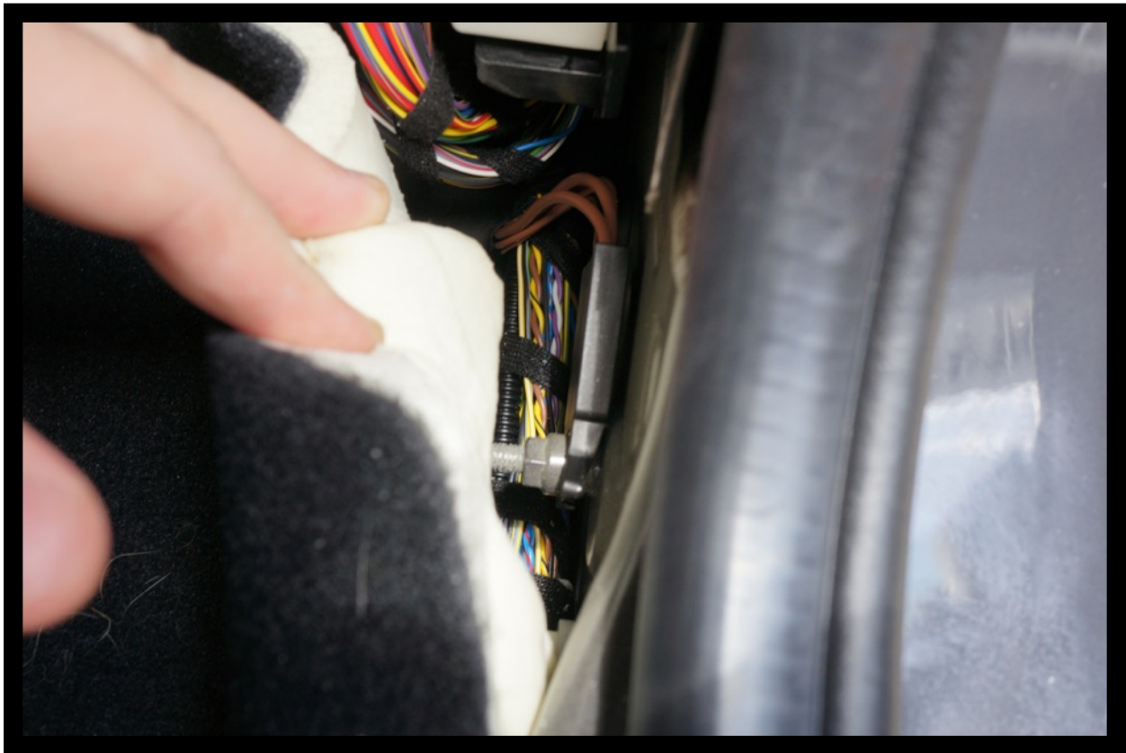
Chassis ground behind the carpet.
