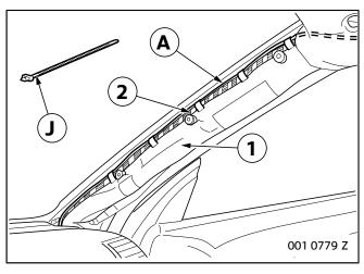
In order to not adversely affect the function of the airbag (1), secure wiring harness **A** to the standard wiring harness (2) with cable tie **J**. ◀
