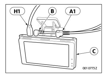
Connect branch **A1**, GPS antenna **B** and branch **H1** (optional) to front camera **C**.
