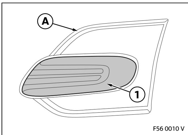
Insert indicator (1) into decorative finisher A and press on firmly until the indicator (1) engages.
