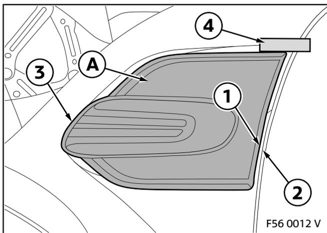
Place decorative finisher A on the wing and position it until the indicator on decorative finisher A is located noticeably low down on the bodywork.
