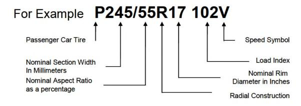
Load Index: a numerical code indicating the maximum load carrying capacity of a tire at the maximum cold inflation pressure.
