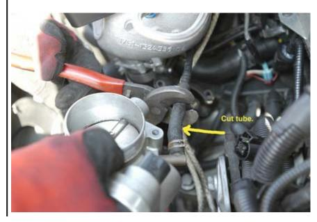
black and gray tubes. We highly recommend using extra long needle nose pliers for this. The black tube needs to be disconnected. To do this, find the quick-disconnect toward the firewall and press the small white tab on the side of the joint. The gray tube is connected to a map sensor. First unbolt (2) #2 Allen screw, now the gray tube can be easily removed.
