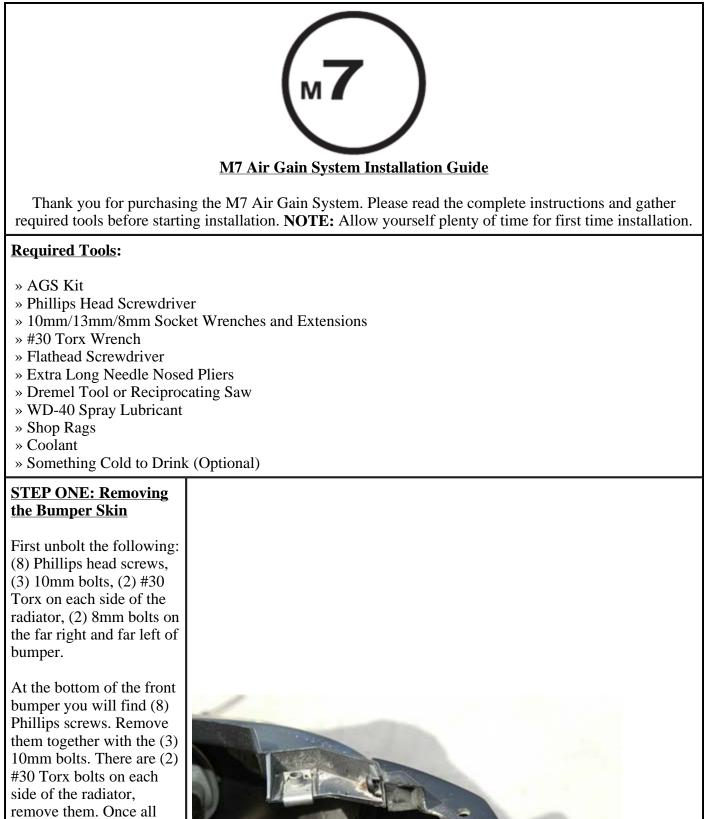
remove them. Once all the bolts are off, reach in and and disconnect the lamp wiring and thermometer wiring. Now remove the front bumper skin off the car.
