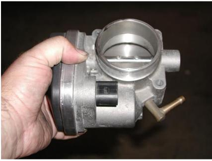
If you have an AGS Pro System with a larger throttle body, just set the stock unit aside, and return it to M7 to get your core charge refunded. If you are going to reuse your stock TB, you must remove the right angle vacuum hose barb and replace it with the low profile connector supplied with your kit. Also, the barb should point to the back side of the throttle body, the side with the rubber gasket.
