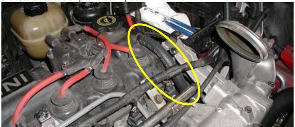
This photo shows the routing on the head. Now you can replace the intercooler. I have found the technique used for removal works pretty good backwards! It takes a bit the first time, but I've found this to be a fast and easy way to get the IC back on. Make sure the IC boot clamps are tight, and don't forget the 8mm bolts that hold the IC supports to the intake manifold. Re-install the cover.
