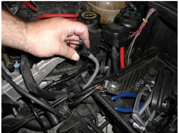
Remove the MAP sensor, and pull out the stock MAP sensor vacuum tube.
