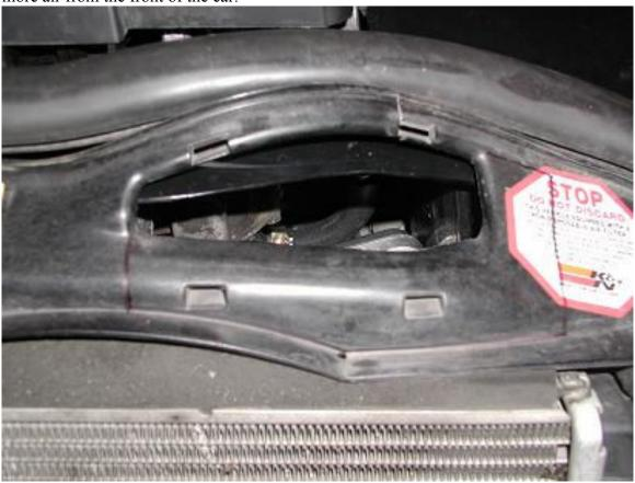
First, mark where you're going to cut. I used a black Sharpie, and stopped my enlargement where there is a bracing rib on the back of the shroud.
