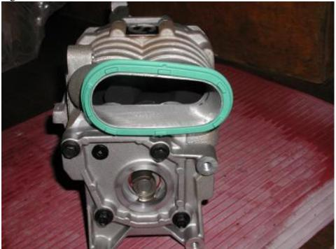
This shows the gasket mounted on the supercharger intake. Note that it's asymmetrical, with one end smaller than the other. There is a rubber alignment tab as well.
