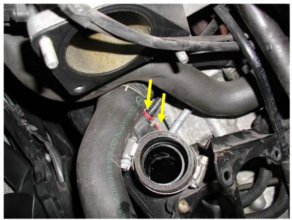
Next, remove the two vacuum lines. If you push down on the red collar, the tube can pull out. The above photo shows the grey tube removed, and the black still in place. Now you can remove the 10 mm nut that attaches the intake duct to the supercharger, and remove the duct from the car. If you chose to not remove the bypass valve assembly, you will have to use long needle nosed pliers to get to the red release collars.
