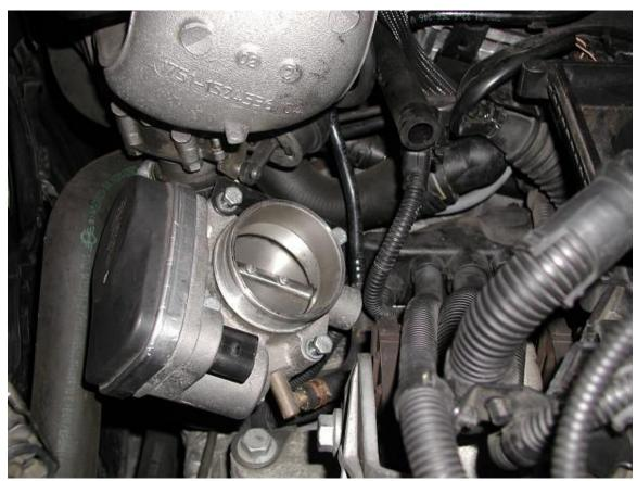
Disconnect the wiring harness (remember these are locking connectors, so make sure you press on the lock enough so that the connector slides off without fighting), the 4 10mm bolts, and the vacuum hose (this last item may be easier to remove after the throttle body is no longer mounted to the car). The clip on the vacuum hose can be moved with pliers. The throttle body is captured between the support bracket and the stock tube. It will come out, but it takes a little coercion!
