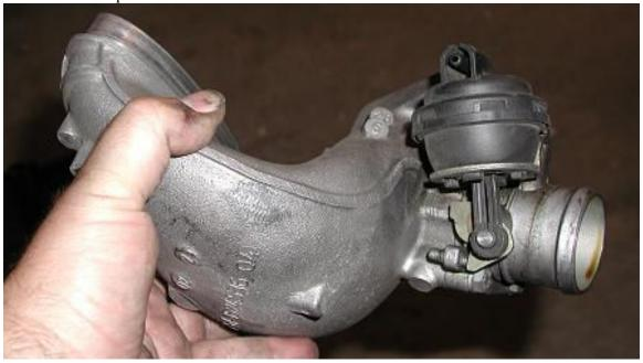
If you've never checked your bypass valve, now is a good time to do so. Make sure that the set screw that limits travel allows the valve to fully close. Also, some valves have needed the butterfly adjusted. Thread lock was used on later model years, so if you're going to make adjustments to your valve, you may have to use some heat to loosen things up.
