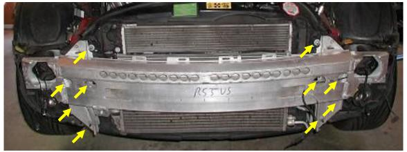
Remove the wires from the brace so they won't get snagged when the brace is removed from the car. Each side is attached with 4 13 mm nuts, and one 13 mm bolt. Remove all 10 of these connectors, and the brace will pull away and off of the car.
