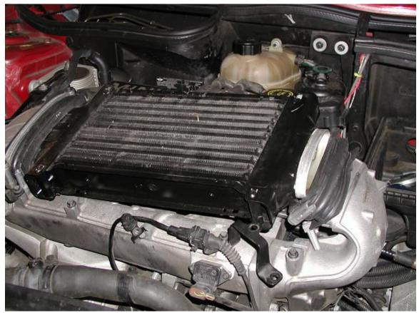
Remove the smaller boot, and the lower half of the three clamps that had been loosened.
