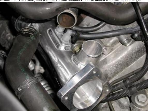
Install the AGS tube, and use the 10 mm shoulder bolt to attach it to the supercharger.
