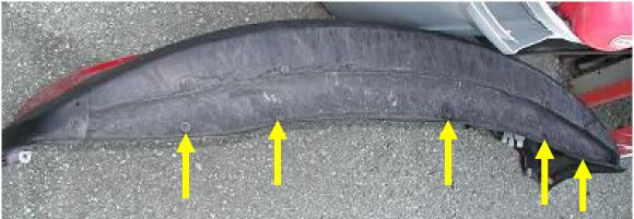
Next, remove the two (one each side) 8 mm bolts from within each wheel well. Long extensions can help here.
