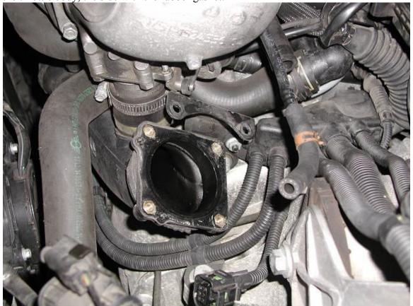
This shows the stock tube that will be replaced. You can also see the bypass valve and the cooling hoses.
