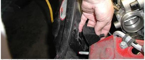
Cut this tab off the radiator shroud. That's the last bit of removal.
