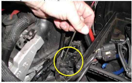
The grey tube you removed in the last step goes to the MAP sensor. It's mounted above the thermostat housing at the end of the head near the air box. The MAP sensor must be removed to fully remove and replace the tube. It's held in place with two 3mm Allen socket head cap screws.
