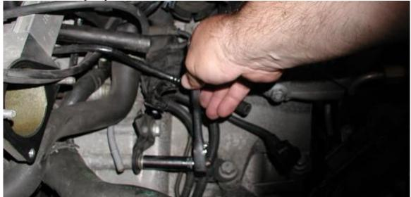
Next, remove the throttle body support bracket. This won't be used in with the AGS system. It's held in place with two 13 mm bolts, and the wiring harness is attached with a 10 mm nut. Disconnect the radiator hose at the water pump. Some coolant will spill, so be prepared.
