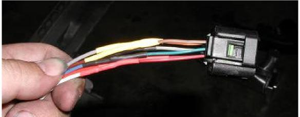
Slide some ½" shrink wrap over the wire bundles (two pieces, one for each end of the splice) so that you can bundle the work after soldering. And remember to put on the small piece of shrink wrap before you solder each wire onto the wiring harness! After all the soldering is done, and the shrink tubing has been hit with a heat gun, add the supplied insulation sheath over the wires. Re-attach the connector cover, and you are done with the wiring!
