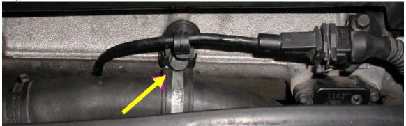
The 10 mm bolt that hold the knock sensor wire and holds the upper radiator hose to the intake manifold must be removed. Now you can lift some of the weight of the MFE, and lean it forward 4-6 inches.
