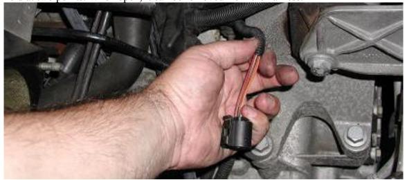
Stretch the wiring sheath back so that you expose enough wire to work with, on both ends! Now comes the hard part. Cut the wires, one at a time. (Cut one at a time in case there is still residual charge built up in the car's electronics.)
