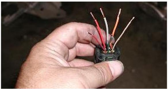
Apply heat and solder to each wire until some solder wicks into the wire. That's it! Now, when you solder the two wires together, all you need to do is heat the solder to re-flow. This takes less time than waiting for the solder to wick as well.
