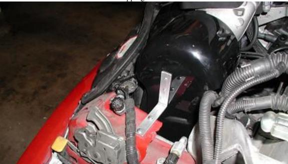
Now is the time to wire-tie the electrical connectors down to the A/C test tube.
