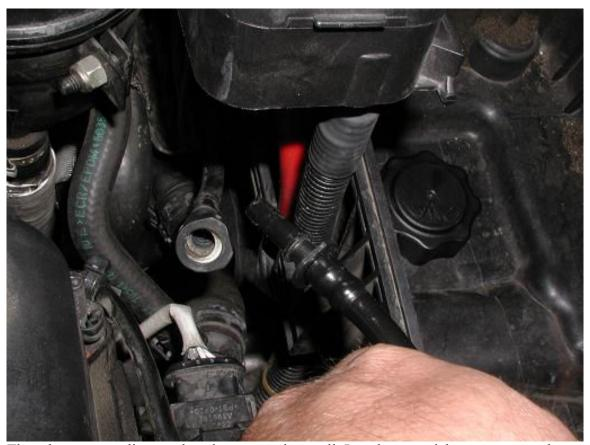
The other vacuum line needs to be removed as well. It ends at a quick connect near the battery terminal. Make sure to press on the white part of the connector to unlock it! When it's disconnected, just pull it out!
