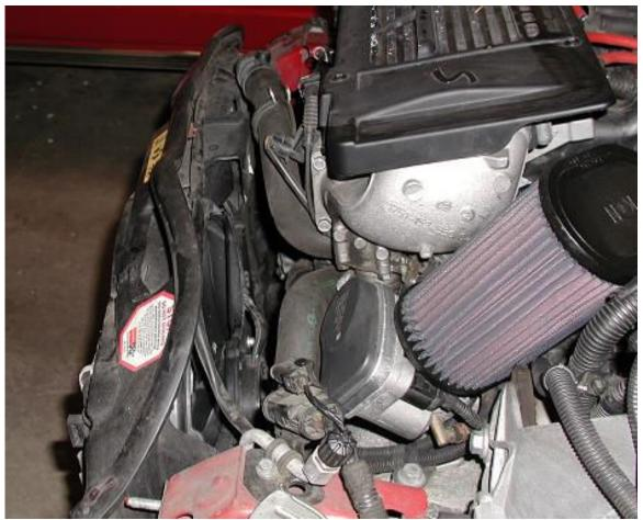
Now there's enough room to work. This is the Hot Air Intake that will be removed to make way for the AGS.
