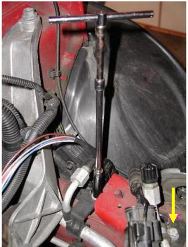
Remove this plastic bracket (held in place with a single 10 mm bolt). Also, slide the round rubber tube protector down. The filter will need the space! Remove the bracket that holds the electrical connectors in place. The electrical connectors will be wire tied in place later.
