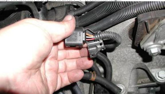
First, remove the cover at the back end of the throttle body connector. It's a snap close
