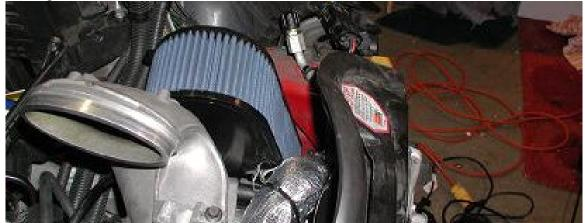
Now's the time to wrap the radiator hose with the insulation, and wire tie it into place.
