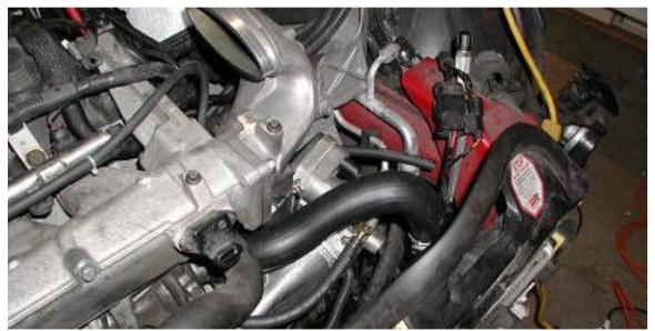
Attach the radiator hose extension included with the AGS kit to the water pump. Mark the stock hose where you will cut it. Cut the hose, and install the coupler with the hose clamps provided. Make sure nothing can rub the TB wiring harness. Note the TB vacuum line now runs above the AGS tube. Route the TB wiring harness under the TB, but don't connect it yet, you'll need the space for putting the filter on.
