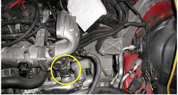
Re-attach the intake horn and bypass valve assembly. Note: The radiator hoses will tuck in tightly. Make sure that the hose clamps for the bypass valve don't restrict the bypass
