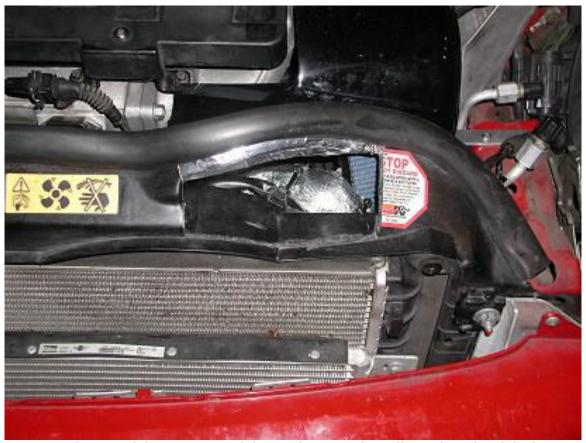
Here I used some Al duct tape to seal the gap between the radiator shroud and the heat shield. Now the AGS will get even more air than stock!
