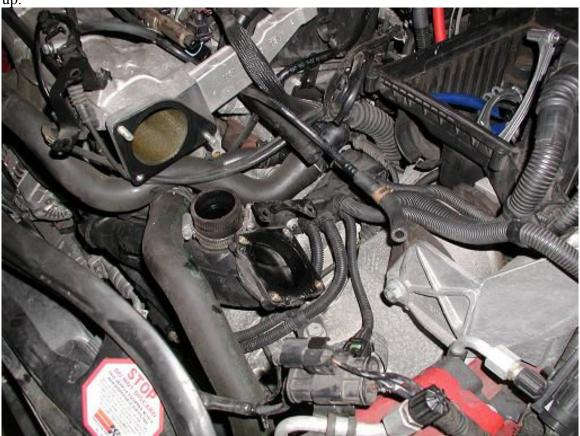
This is the engine bay with the intake, intercooler, throttle body and intake horn all removed from the car.
