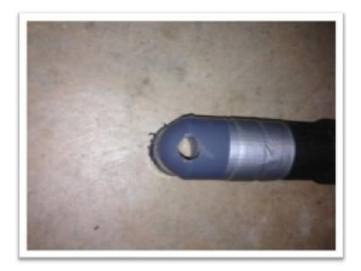
7. The "flange" below is held to the cylinder you are planning to clean by the same nuts that hold the intake manifold in place. You need some air inlet for the vacuum to get its air, so don't worry about a gasket or getting a tight seal.
