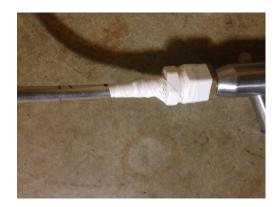
I had planned on making a more professional tool but noted that with a few wraps of electrical tape on the wand extension tubing it would fit snugly inside of the ¼" female pipe thread of the bushing. Time was running short so I used the tape and wrapped the outside of the joint too as shown.
